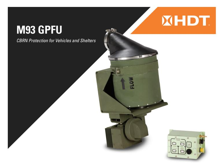
Designed to remove toxic chemical and biological warfare agents in gaseous (vapor) and aerosol (particulate) forms from the airstream, the 100 CFM (170 m3/h) Gas Particulate Filter Unit provides a toxic-free environment to personnel or equipment by creating positive pressure in the toxic-free area (TFA).
