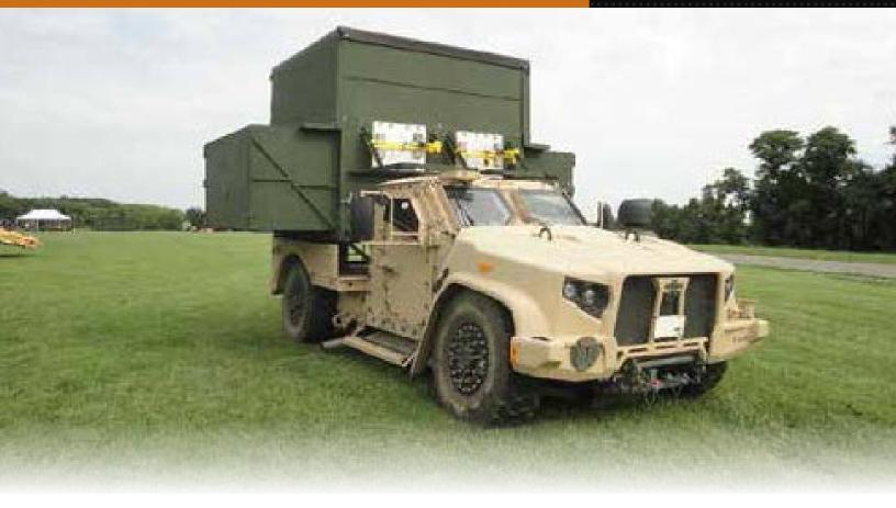
The Joint Light Tactical Shelter (JLTS) provides a mobile shelter solution specifically designed for the Joint Light Tactical Vehicle (JLTV).
