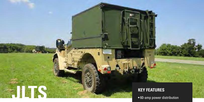
The Joint Light Tactical Shelter (JLTS) delivers a state-of-the-art mobile shelter solution, purpose-built for the Joint Light Tactical Vehicle (JLTV). Featuring lightweight yet robust composite walls, the JLTS is engineered for both durability and operational efficiency, with an expandable design that enhances adaptability across a wide range of mission scenarios.
