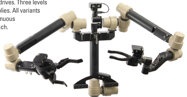
MK4 dual arm system, capable of lifting over 180 pounds (80 kg).
