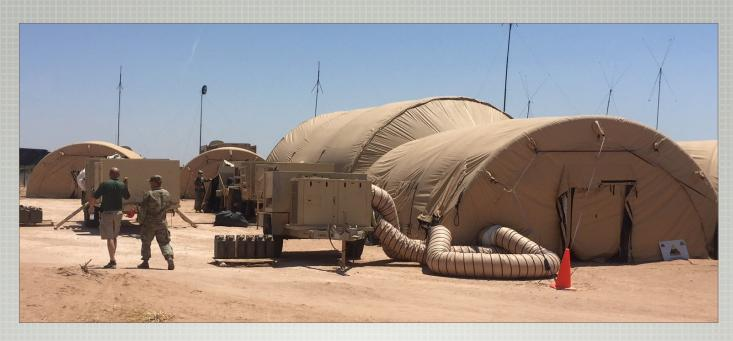
HDT Global's Trailer Mounted Support Systems (TMSS) combine shelter, utilities, environmental control, power and tactical mobility to form a complete command operation center.
