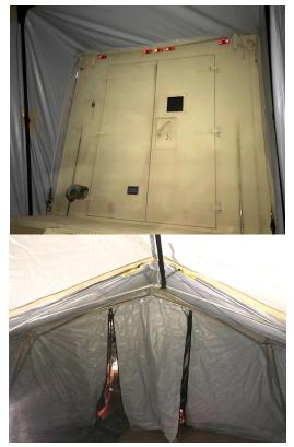
The HDT Expando Van boot weather seal keeps the passageway and occupants dry.
