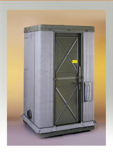
The M14 is a ventilated airlock through which people enter and exit the protected air while airborne hazard is present outside the shelter. The airlock is purged by the flow of clean air. The air flows from the main protected enclosure, through the airlock, and out a discharge vent on the outer airlock door.
