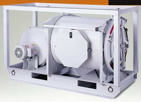
HDT's FFA580-100 is designed to remove toxic chemical and biological warfare agents in gaseous (vapor) and aerosol (particulate) forms from the airstream, while providing a toxic-free environment to personnel or equipment by creating positive pressure in the toxic-free area (TFA). Ideal for mobile or permanent shelters.
