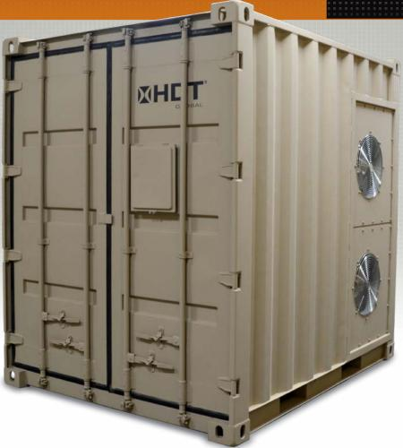
The HDT Containerized Ice Making System (CIMS) is a tricon-style, expeditionary-grade military containerized ice plant that makes 3,600 pounds (1632.9 kg) of ice per day at 120°F (48.9°C) ambient conditions. Built to operate in extreme environments, CIMS only requires water and power to make ice. The system generates ice, then bags the ice, seals the bags, and stores 30 to 60 ten-pound (4.5 kg) bags internally.
