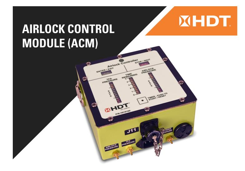
The HDT Airlock Control Module (ACM) is a digital, fully-automated controller that displays the status of the shelter airlock and the toxic-free area (TFA) connected to the airlock. It also displays the required purge time and provides alarms and directions for the airlock occupants. The ACM utilizes the airlock pressure cycles and standard airlock operating procedures to set and reset the purge timer and provide operations instructions to the airlock occupant.
