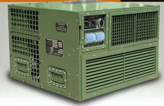
The HDT E2CU-18K is part of the next generation of Enhanced ECU's (E2CU's). The E2CU-18K delivers 18,000 BTU/H (2.6 kW) at 130°F (51.6°C) using the environmentally acceptable refrigerant R-410A. The E2CU delivers Energy Efficiency Ratings (EERs) 20% or more higher than the current ECU's available in the market (as measured in BTU/W). It is designed to the USMC-Enhanced Environmental Control Units (E2CU) interface and performance requirements.
