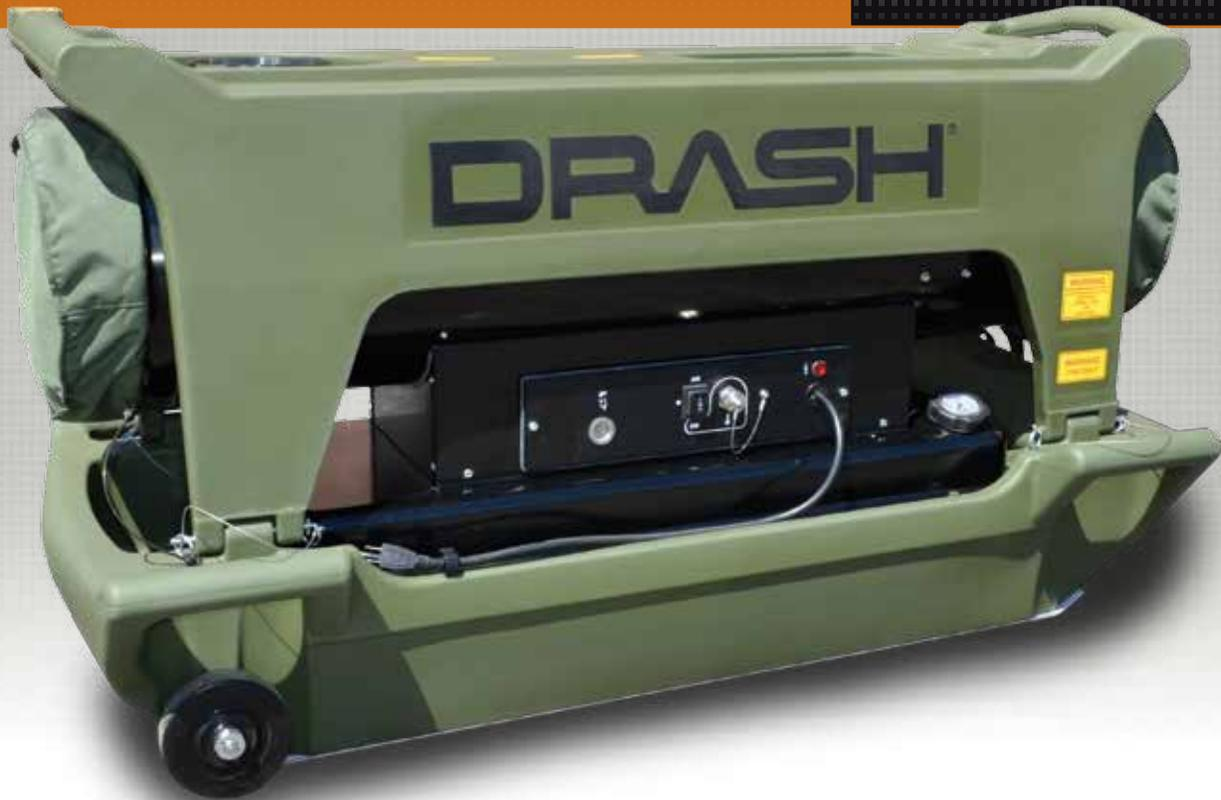
The D-1000B Heater is rugged, lightweight, rust resistant, shockproof and easy to operate and maintain, providing 99,500 BTU/H of dry, clean heat at a rate of 880 CFM (1495 m<sup>3</sup>/h). The heater includes an electronic control system that monitors for high heat conditions and flameout, and operates on an external input of 120 VAC / 60 Hz or 230 VAC / 50 Hz, single-phase power.
