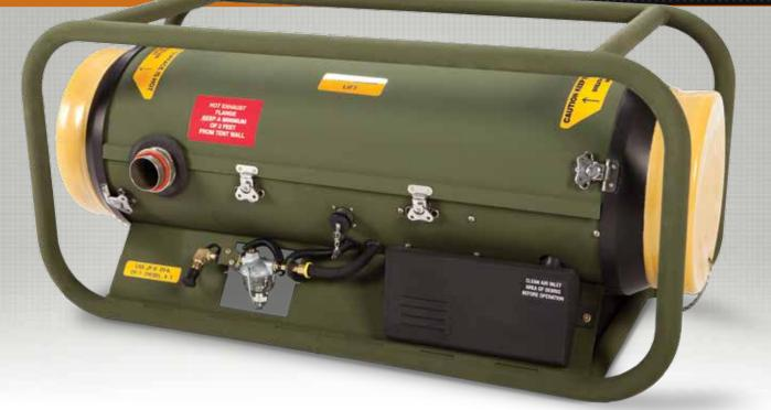
The HDT MTH35 is a self-powered, liquid fuel burning, and ducted convective heater. A thermoelectric generator supplies power for combustion and air handling. Built for optimum efficiency and reliability in strategic field operations, the MTH35 is designed to deliver 300 CFM of clean, heated air to personnel shelters.
