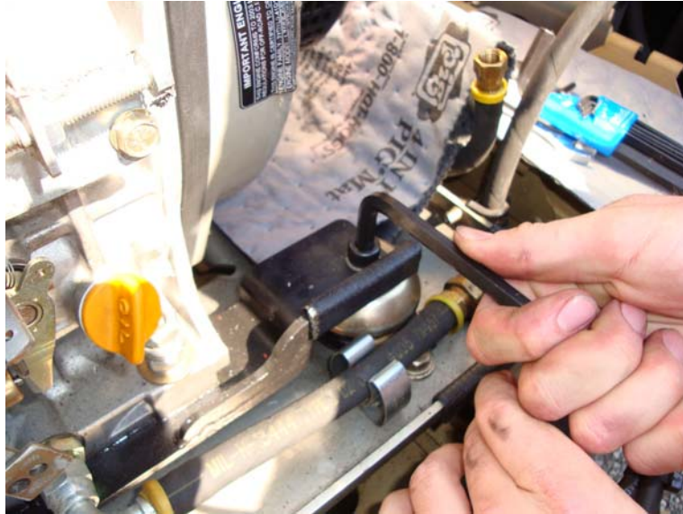
Figure 20. Remove Socket Cap Head Screws Securing Engine Mounting Bracket to Vibration Mounts.
