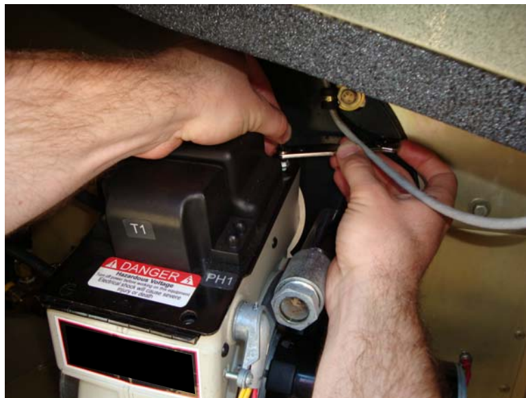
Figure 12. Position Ignition Assembly on Burner Housing and Secure with Screws.
