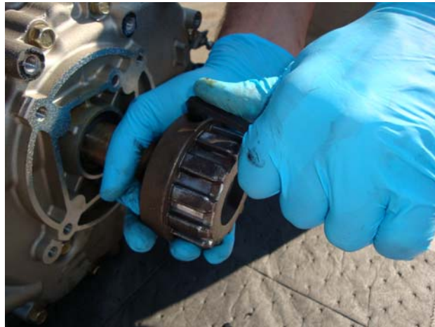
Figure 32. Loosen the Coupler Grip on Engine Shaft.
