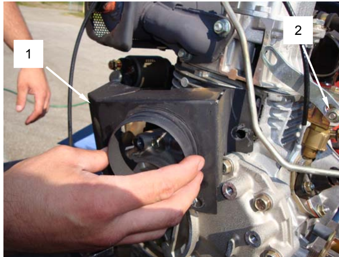
Figure 24. Remove Engine Head Cooling Air Inlet Box.
