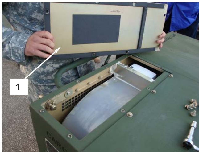
Figure 1. Removing the Carbon Monoxide Detector Cabinet Cover.
