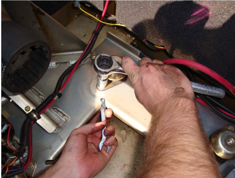
Figure 26. Removing Defective Vibration Mount.
