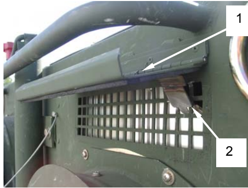
Figure 15. Operating the Fresh Air Damper.
