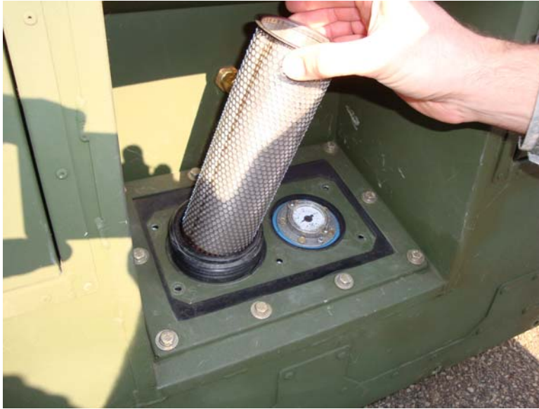
Figure 2. Remove Fuel Filler Cap and Strainer.
