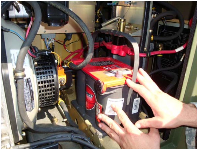
Figure 65. Install Battery Farthest from Access Door.
