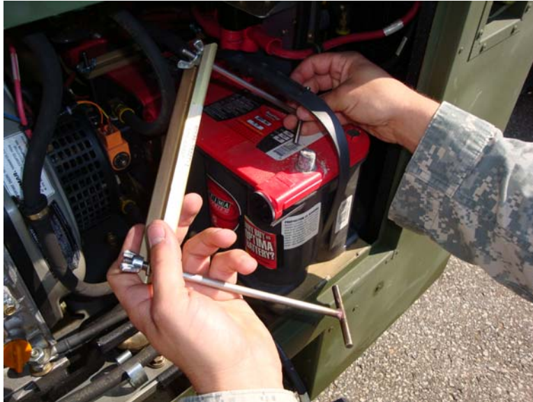
Figure 5. Remove Battery Hold-down Bracket.
