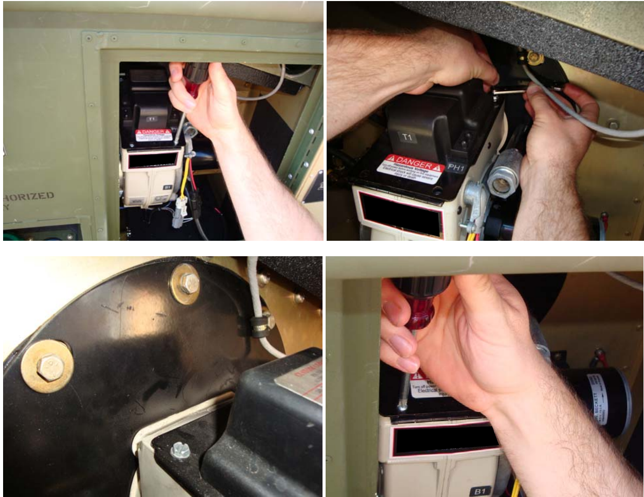
Figure 1. Remove Screws Securing Ignition Assembly.
