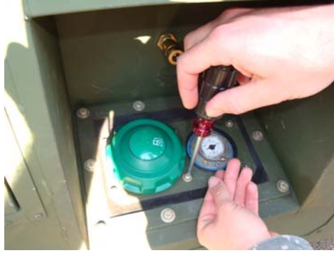
Figure 1. Removing Hardware Securing Retaining Plate.
