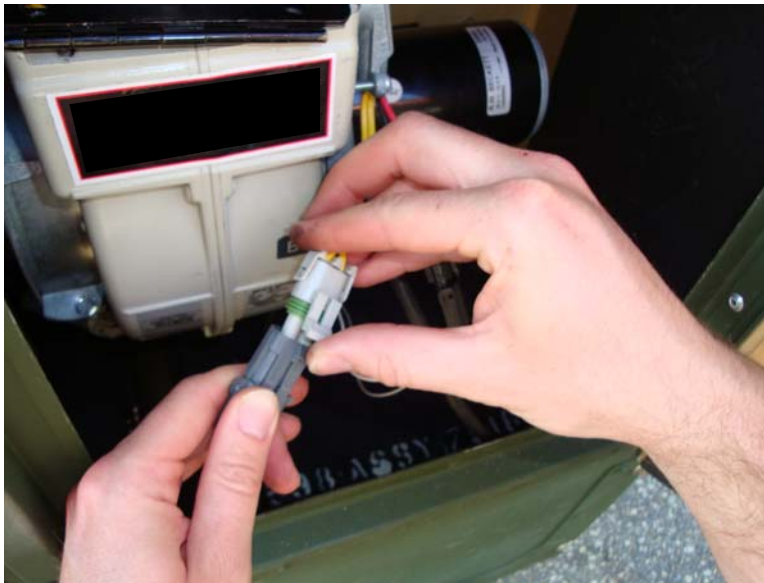
Figure 8. Disconnect Flame Sensor Connector.
