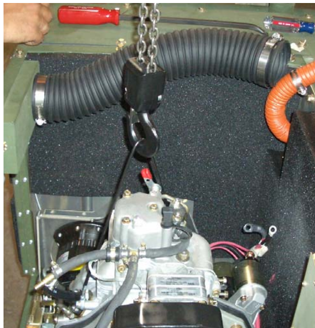
Figure 23. Attach Chain Lift to Engine Lifting Cable.
