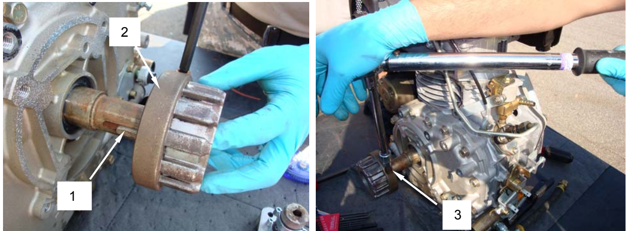
Figure 39. Install Coupling Hub on Drive Shaft.
