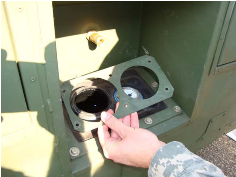
Figure 11. Position Retaining Plate Over Fuel Tank Filler Neck and Fuel Gauge.
