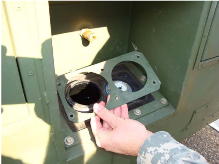
Figure 3. Remove Retaining Plate.
