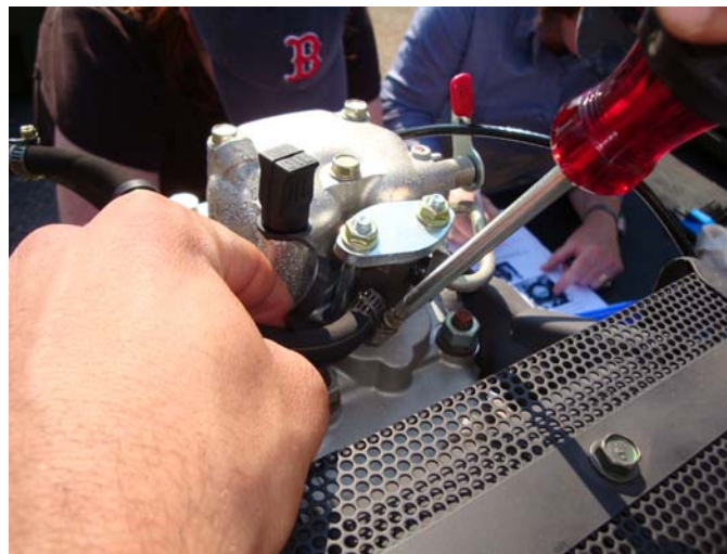
Figure 25. Remove Fuel Hose from Fuel Injector Pump.
