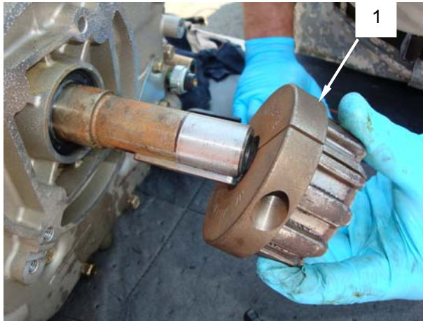
Figure 33. Remove Coupling Hub and Rubber Coupling (if attached).
