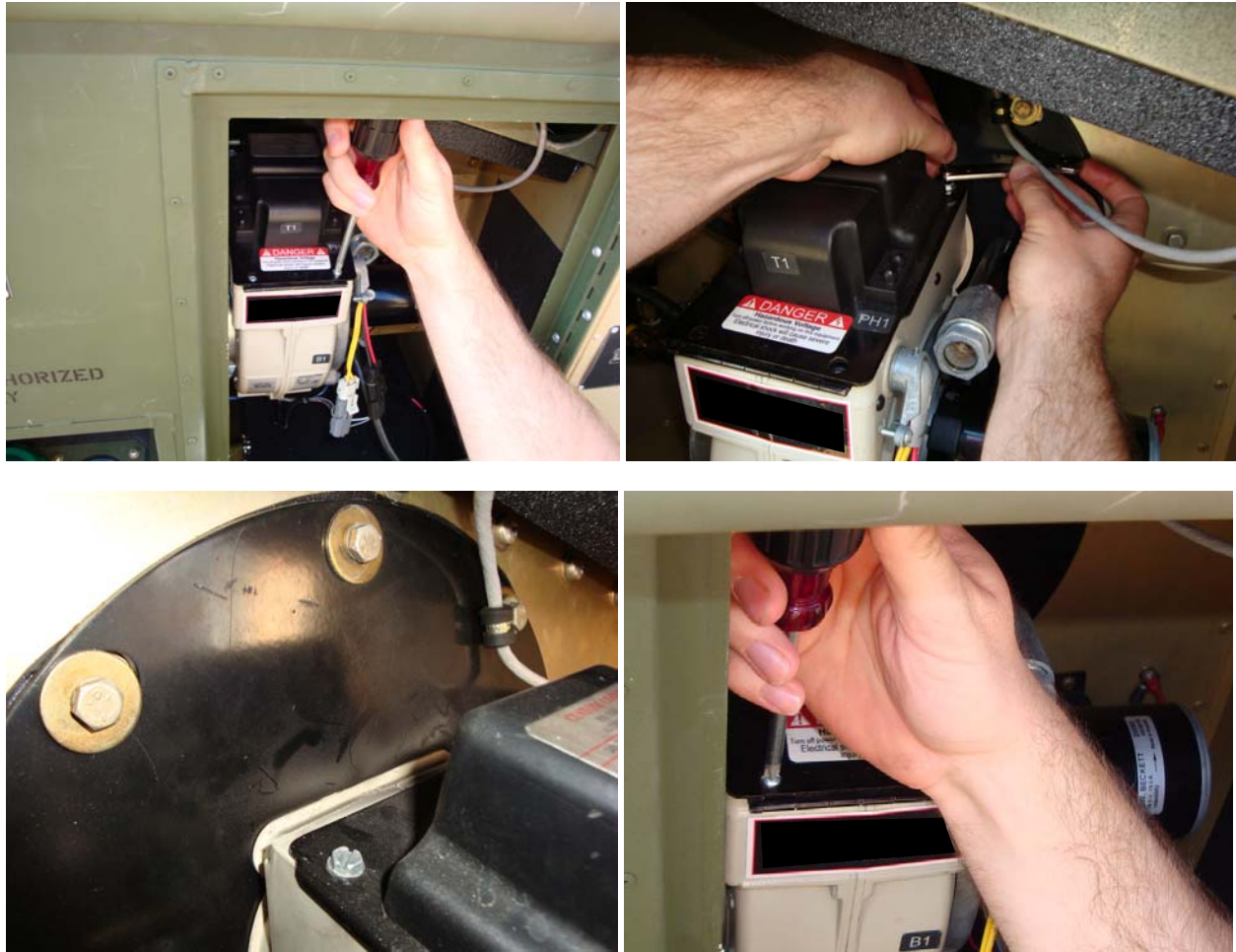
Figure 14. Remove Screws Securing Ignition Assembly.
