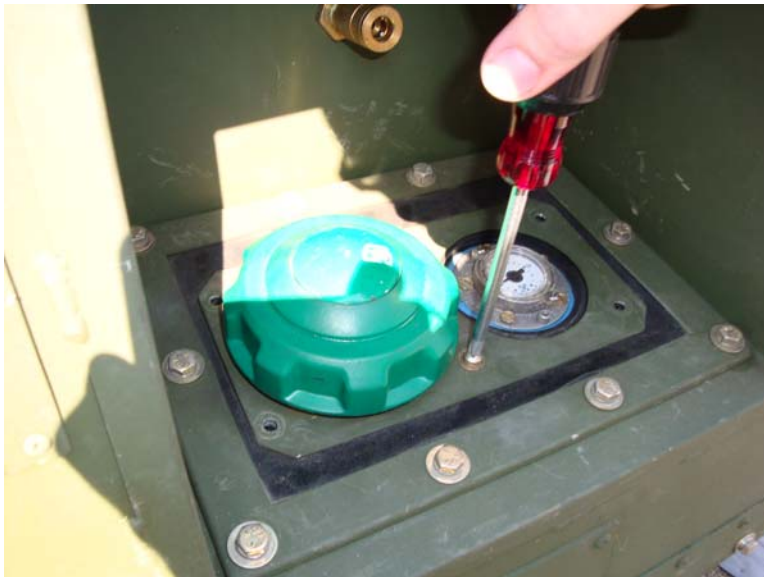
Figure 25. Install Hardware to Secure Retaining Plate.
