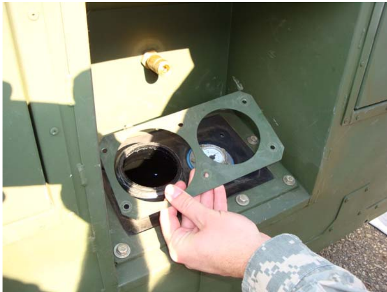
Figure 3. Remove Retaining Plate.
