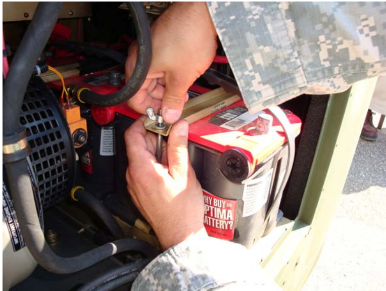
Figure 4. Remove Hardware Securing Battery T-bar Closest to Access Door.
