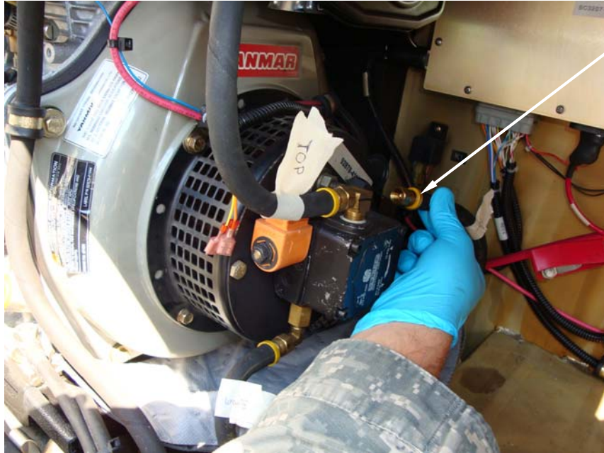
Figure 13. Remove Fuel Hose at Back of Burner Fuel Pump.
