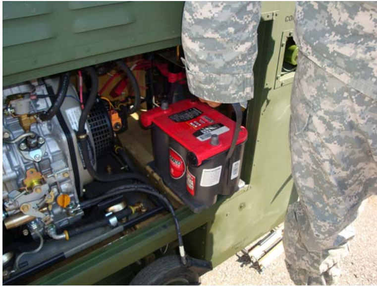
Figure 10. Remove Battery Farthest from Access Door.
