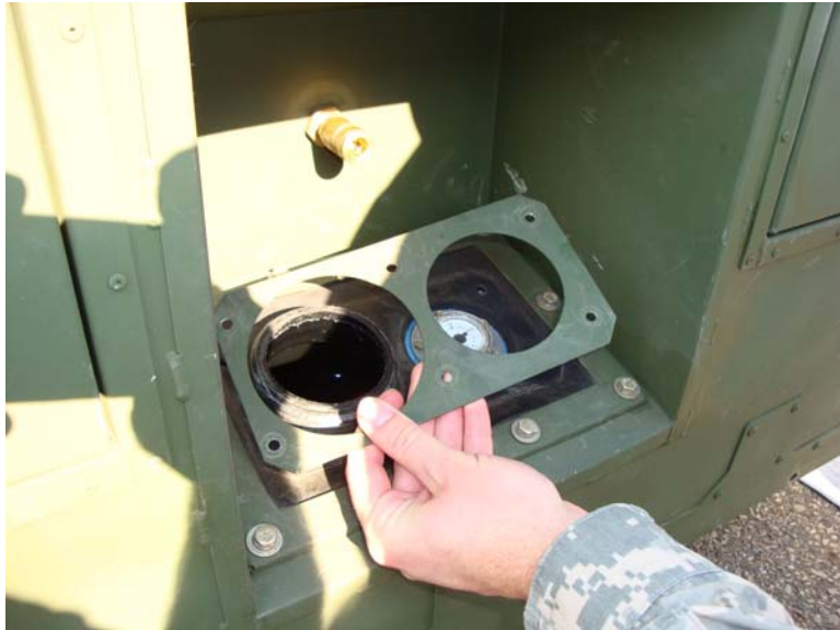
Figure 3. Remove Retaining Plate.
