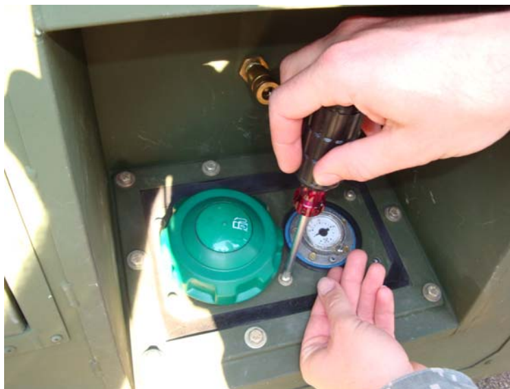
Figure 1. Removing Hardware Securing Retaining Plate.
