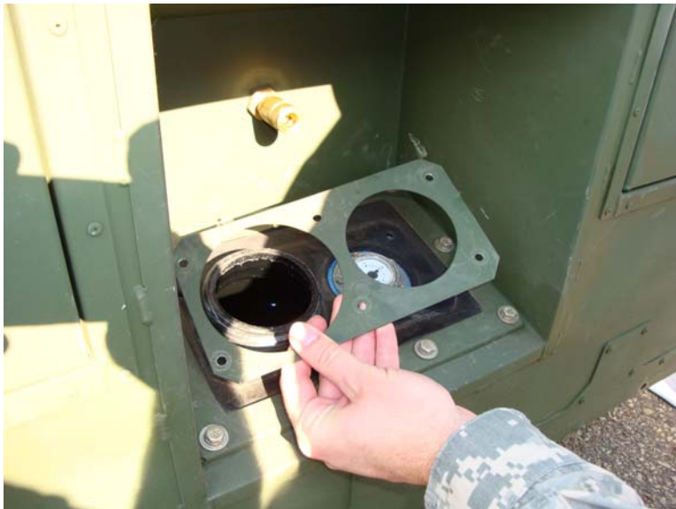
Figure 23. Position Retaining Plate Over Fuel Tank Filler Neck and Fuel Gauge.
