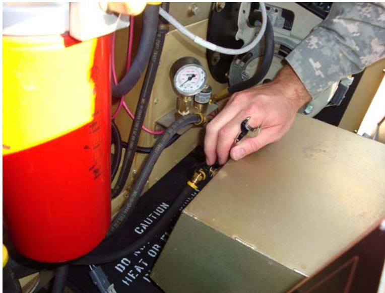
Figure 10. Install External Fuel Hose to Fitting.
