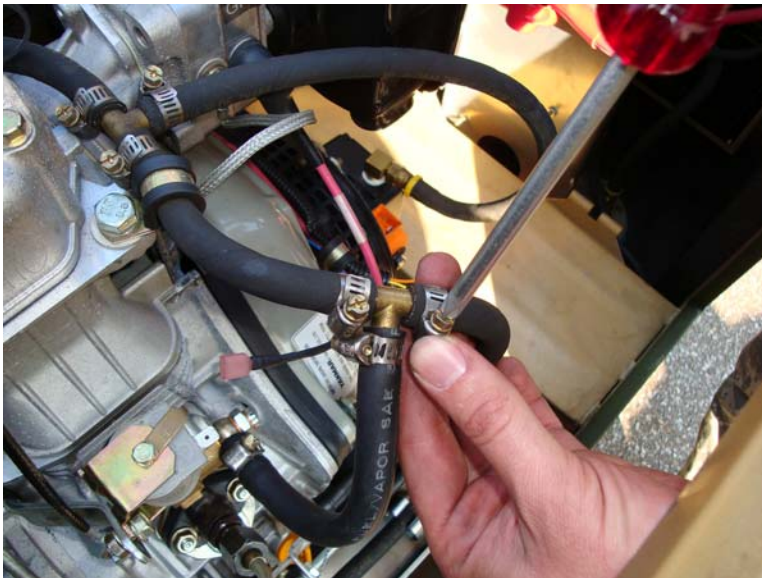
Figure 61. Connect Fuel Supply Hose to Arm of Tee Connector.
