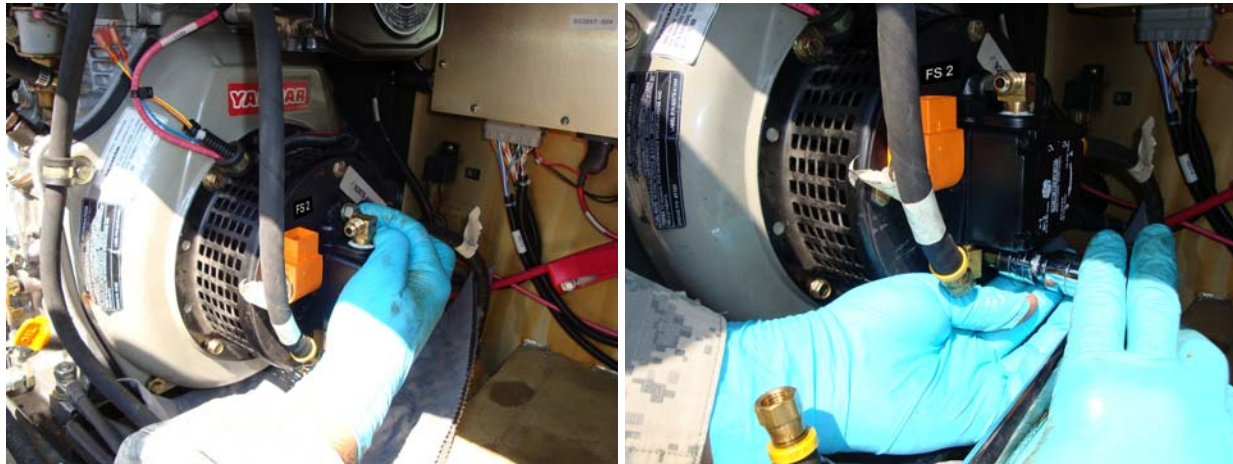
Figure 20. Secure Burner Fuel Pump to Flywheel Cover.
