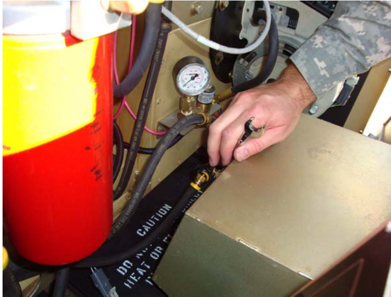
Figure 22. Install External Fuel Hose to Fitting.
