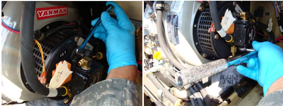
Figure 16. Remove Hardware Securing Burner Fuel Pump to Flywheel Cover.
