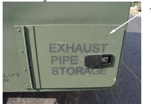
Figure 19. Exhaust Stack Stowage Area.
