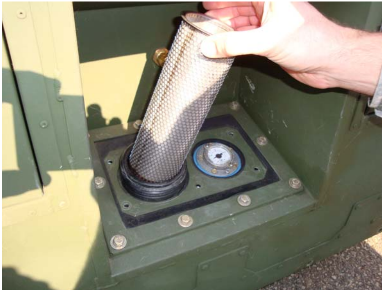
Figure 2. Remove Fuel Filler Cap and Strainer.
