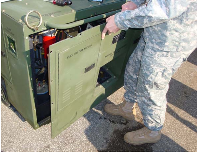
Figure 9. Move End Panel into Position Near Fuel Tank.
