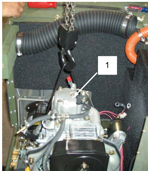
Figure 22. Attach Chain Lift to Engine Lifting Cable.
