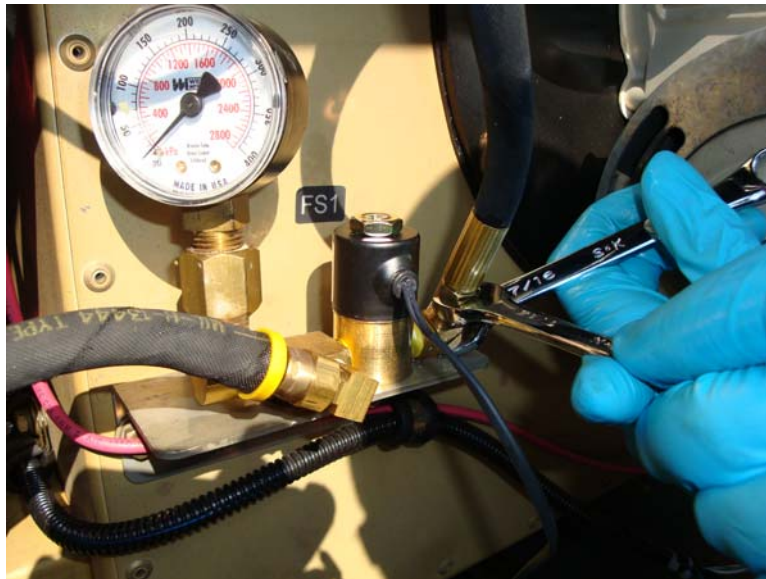
Figure 19. Install Burner Feed Line on Elbow Fitting.
