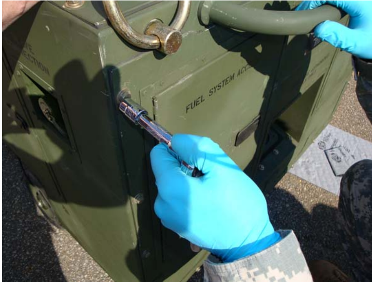
Figure 4. Remove Hardware from Perimeter of End Panel.
