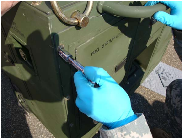
Figure 12. Install Hardware Around Perimeter of End Panel.
