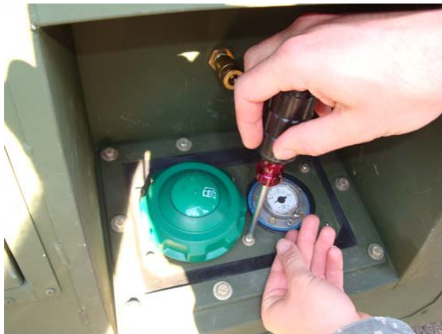
Figure 1. Removing Hardware Securing Retaining Plate.
