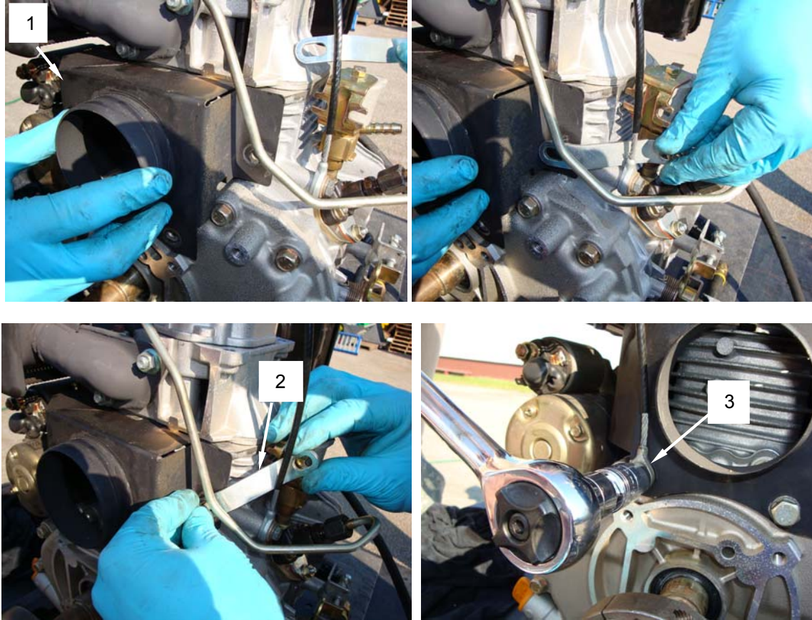
Figure 45. Install Engine Head Cooling Air Inlet Box.
