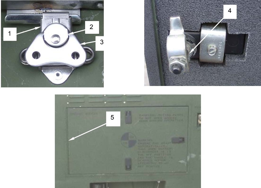
Figure 1. Lubricate All Latches and Hinges.
