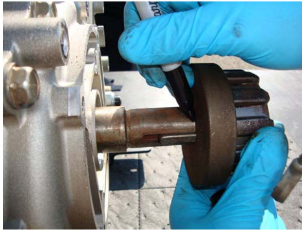
Figure 31. Mark the Engine Shaft.
