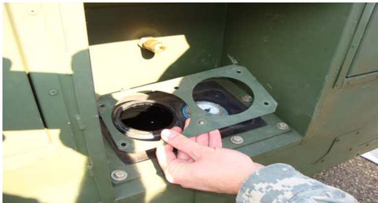
Figure 3. Remove Retaining Plate.
