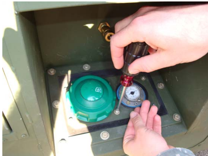
Figure 1. Removing Hardware Securing Retaining Plate.
