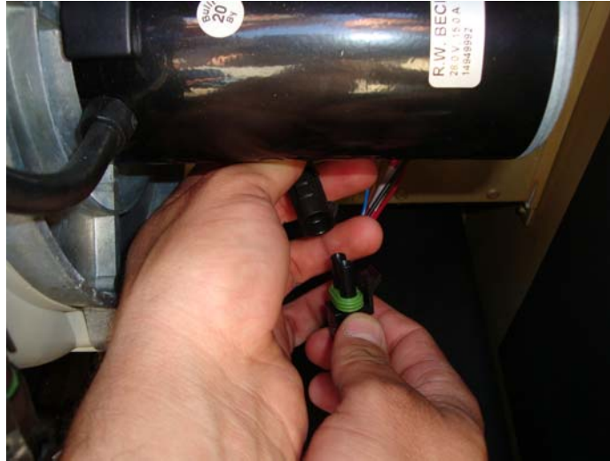
Figure 1. Disconnect Combustion Blower Wiring Harness Connector.
