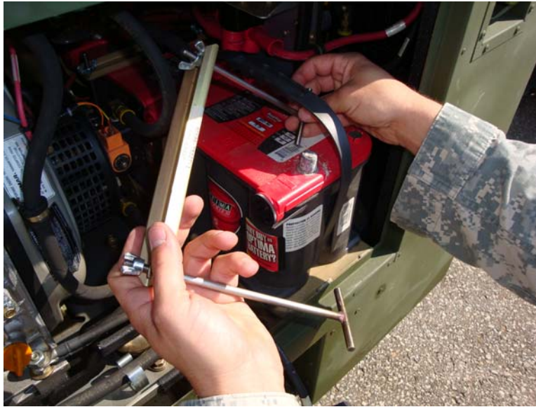
Figure 5. Remove Battery Hold-down Bracket.
