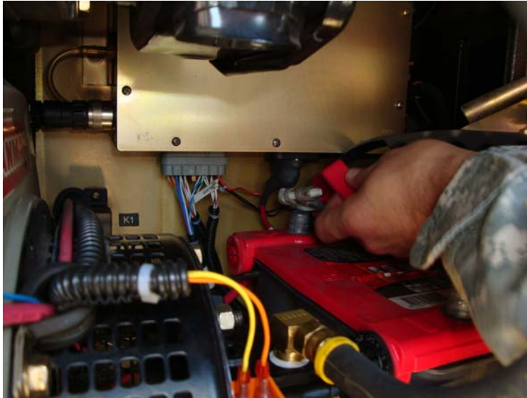
Figure 9. Remove Positive Battery Cable of Battery Farthest from Access Door.
