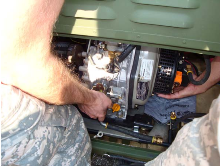
Figure 24. Remove Engine from Heater.
