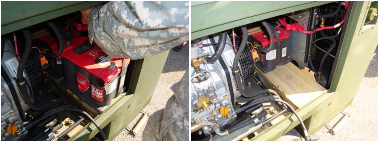
Figure 6. Remove Battery Closest to Engine Access Door.
