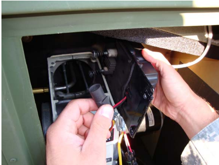
Figure 3. Remove Flame Sensor Bracket from Slot on Ignition Transformer.
