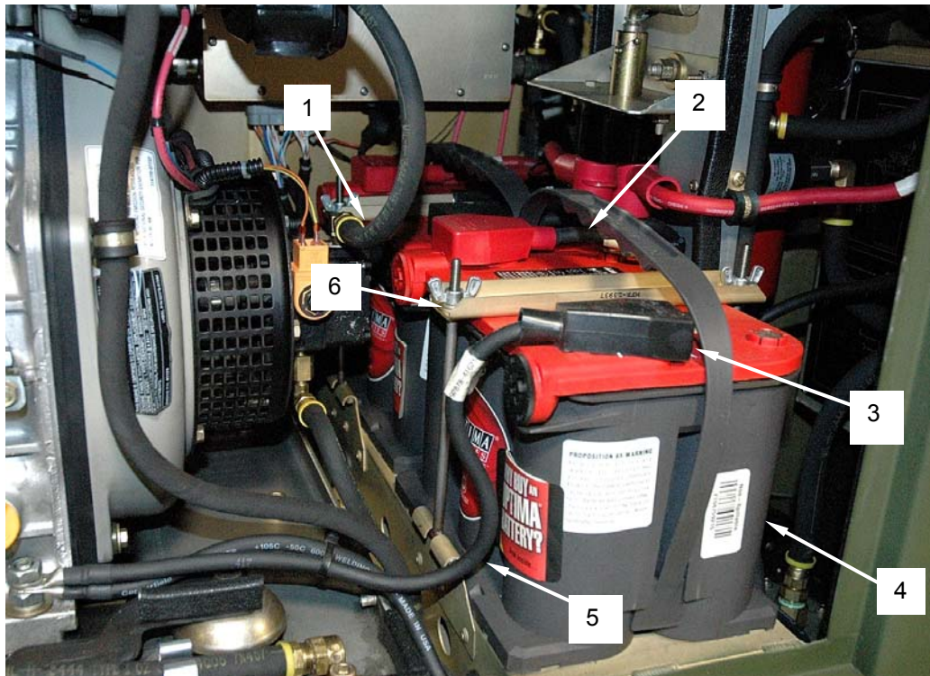
Figure 3. Before and After Operation PMCS for Batteries.
