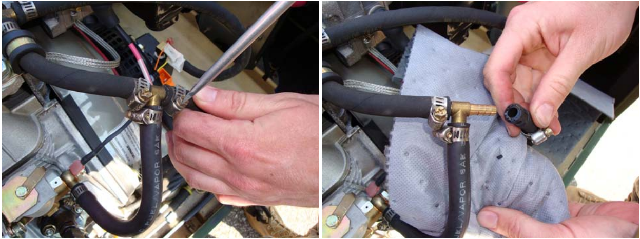
Figure 14. Remove Fuel Supply Hose from Arm of Tee Connector.
