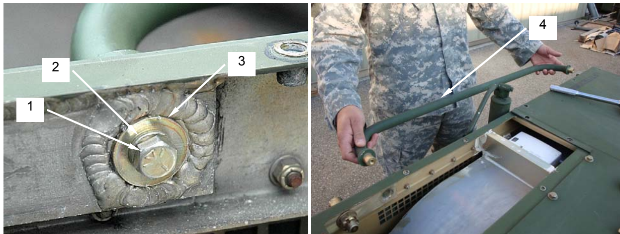
Figure 3. Removing the Damaged Mobility Handle.
