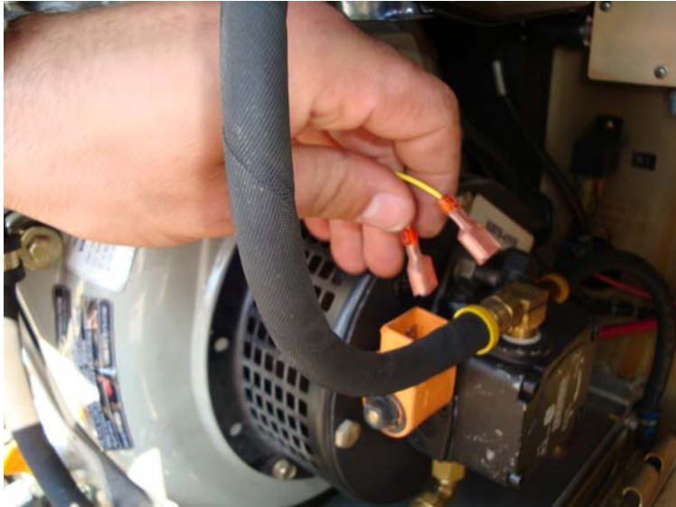
Figure 11. Remove Wires Connected to Burner Fuel Pump.
