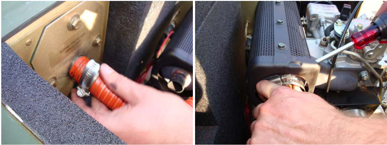
Figure 64. Install New Flexible Exhaust Tube.
