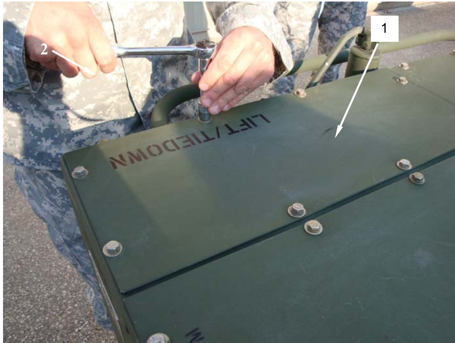
Figure 6. Installing the Covers on the Cabinet.
