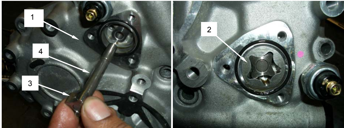
Figure 3. Inspect Oil Pump.
