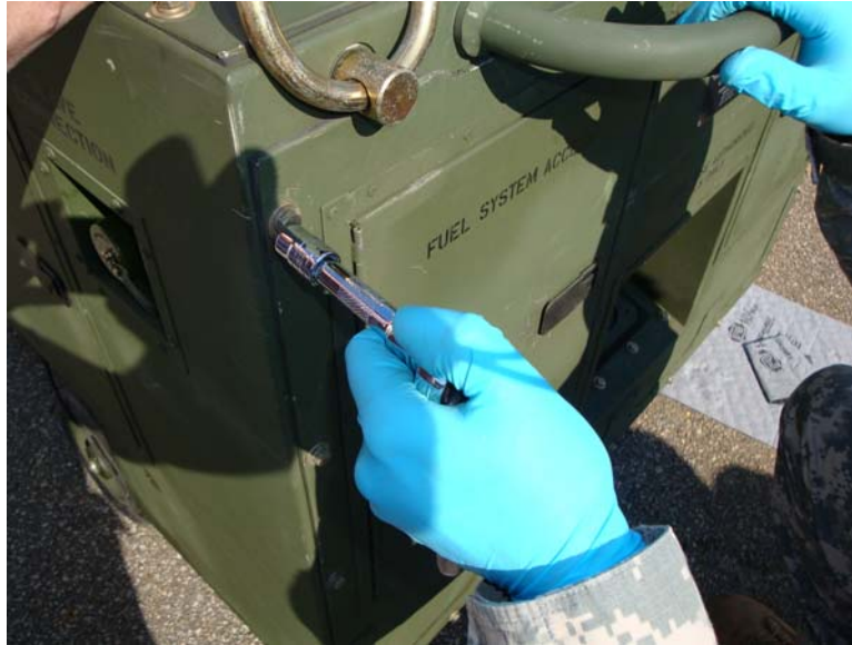
Figure 4. Remove Hardware from Perimeter of End Panel.
