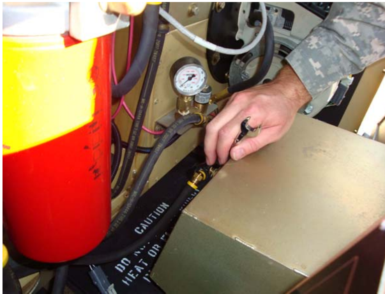
Figure 10. Install External Fuel Hose to Fitting.
