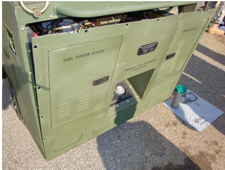
Figure 5. Move End Panel from Heater to Gain Access.
