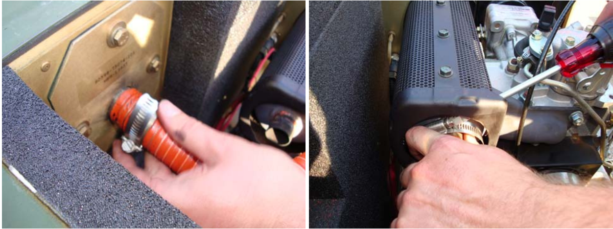
Figure 44. Connect Flexible Exhaust Tube to Engine Muffler.
