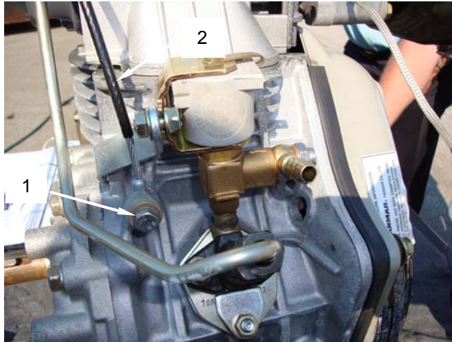
Figure 37. Remove Lift Cable.
