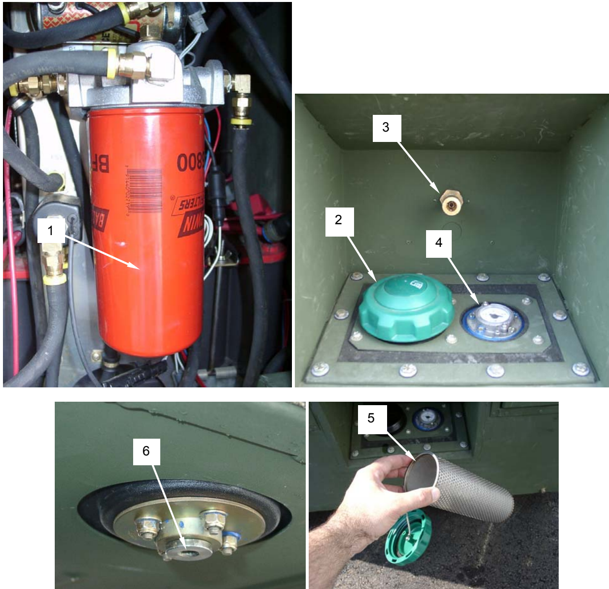
Figure 2. Fuel System Controls and Indicators.
