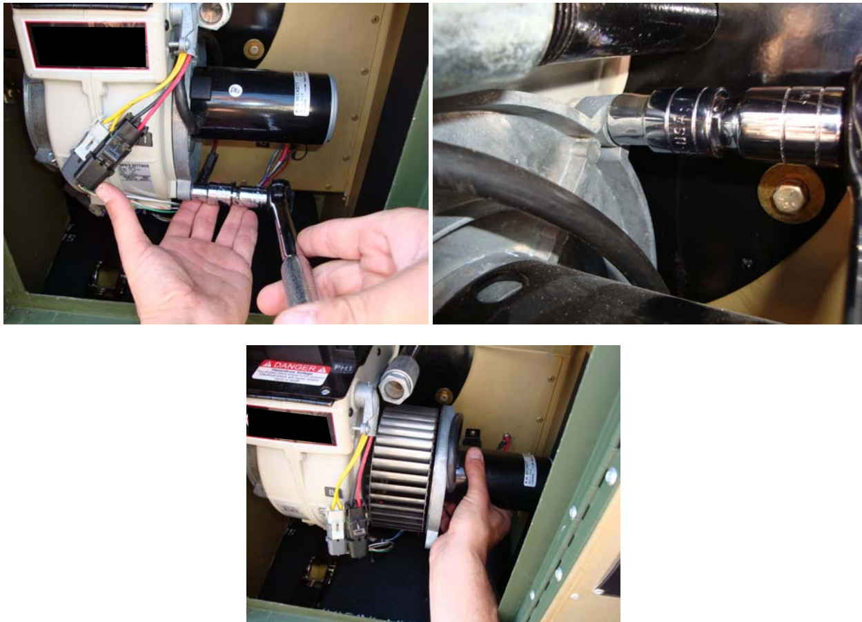
Figure 2. Remove Combustion Blower from Burner Housing.
