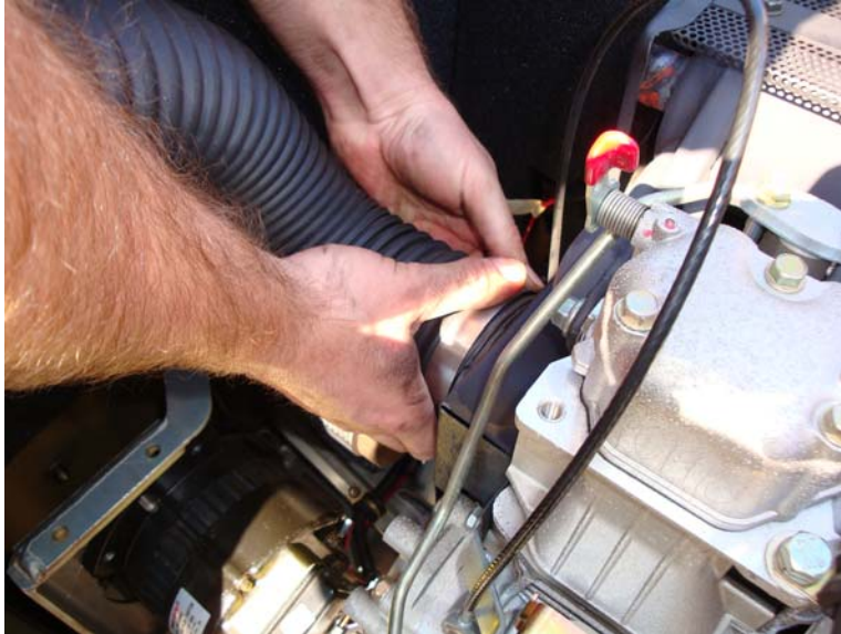
Figure 21. Remove Engine Header Exhaust Hose.
