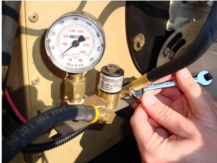
Figure 8. Remove Burner Feed Line from Elbow Fitting.
