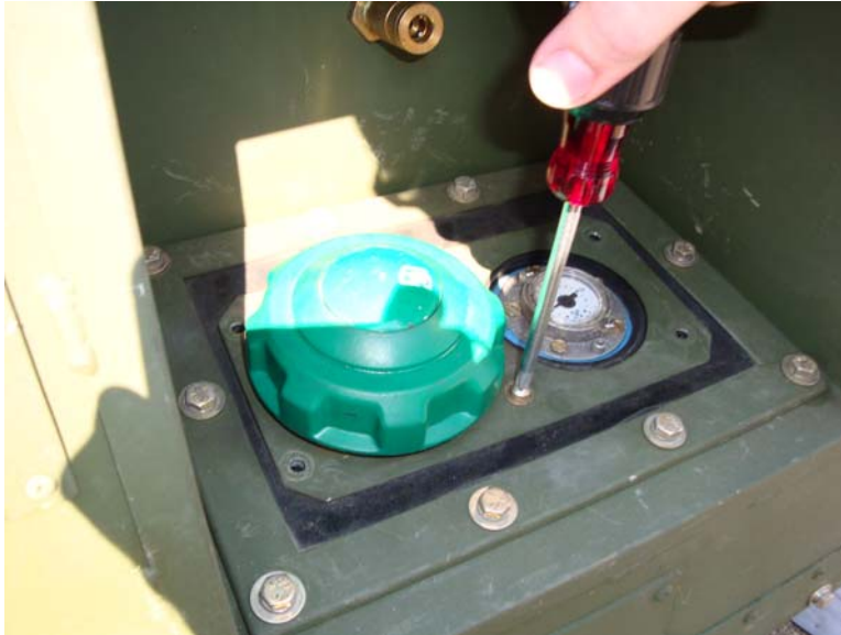
Figure 13. Install Hardware to Secure Retaining Plate.
