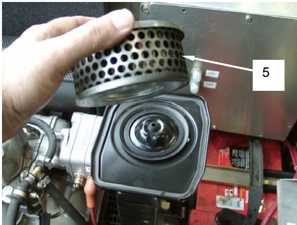
Figure 1. Inspect and Replace Filter Element.
