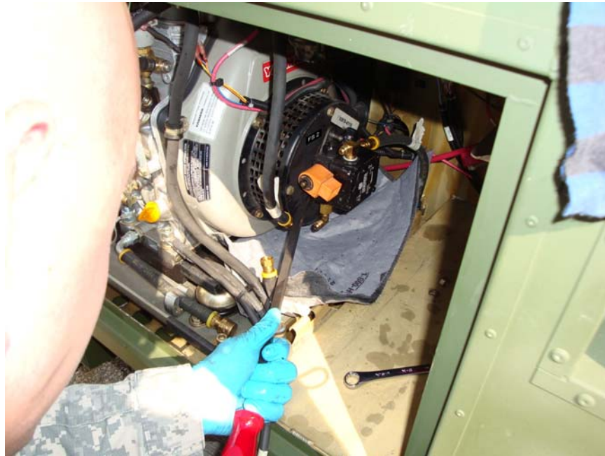
Figure 17. Remove Burner Fuel Pump from Flywheel Cover.
