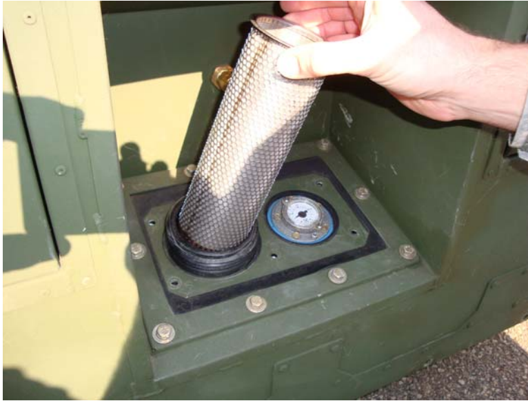
Figure 2. Remove Fuel Filler Cap and Strainer.
