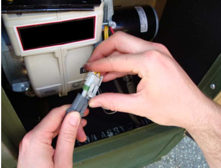
Figure 11. Reconnect Flame Sensor Connector.
