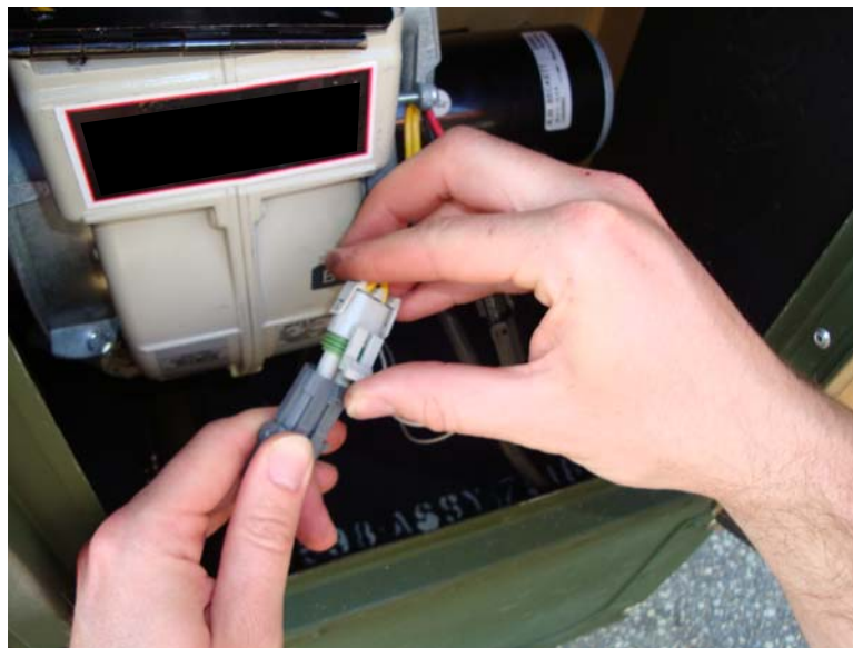
Figure 19. Reconnect Flame Sensor Connector.
