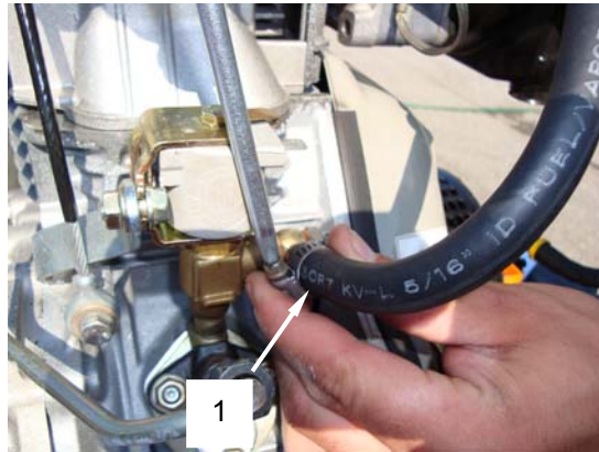
Figure 26. Remove Hose from Engine Shutdown Solenoid Fitting.
