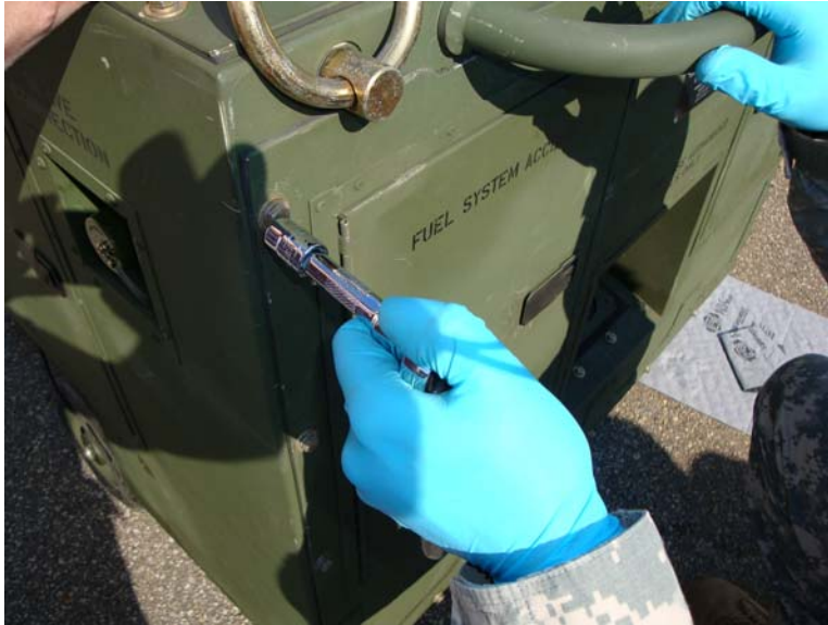
Figure 24. Install Hardware Around Perimeter of End Panel.
