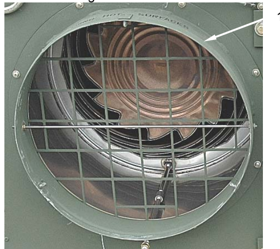
Figure 11. Heated Air Outlet.
