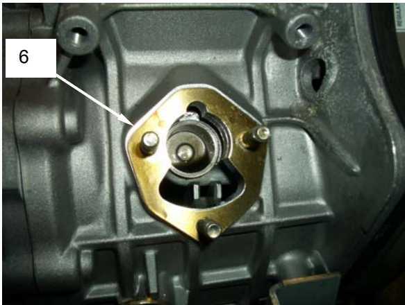
Figure 4. Fuel Injection Timing Adjustment.
