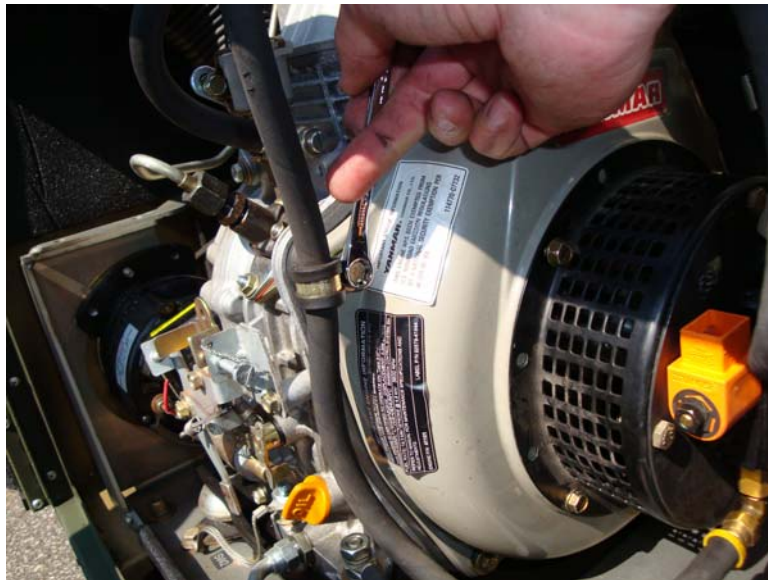
Figure 15. Remove Clamp Securing Fuel Supply Hose to Engine Flywheel Housing.
