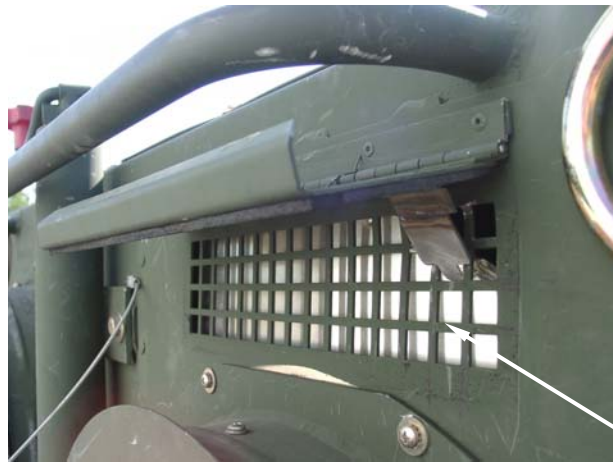
Figure 12. Fresh Air Damper.
