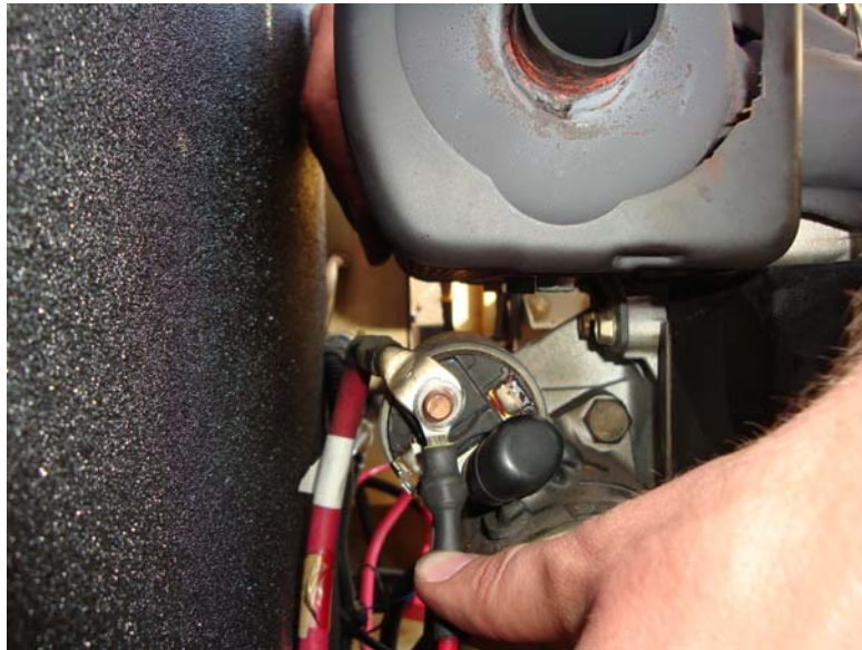
Figure 43. Connect Wires to Starter Solenoid.
