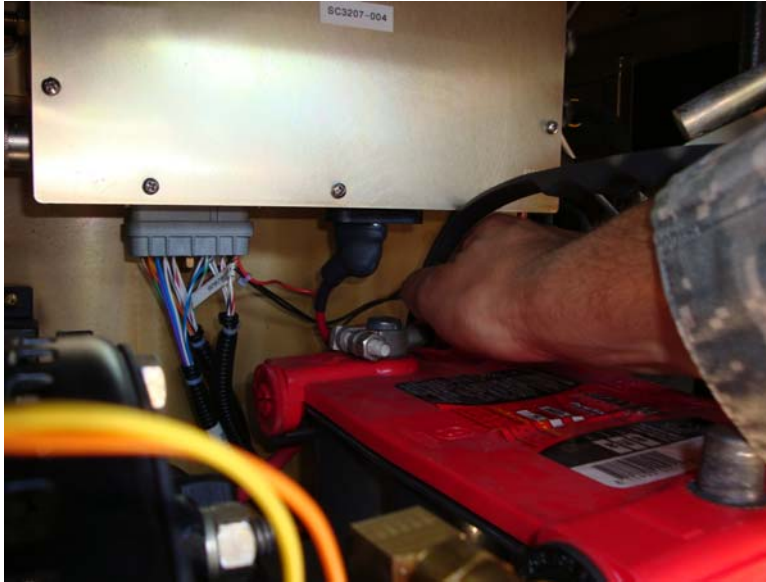
Figure 46. Install Positive Battery Terminal of Battery Farthest from Access Door.
