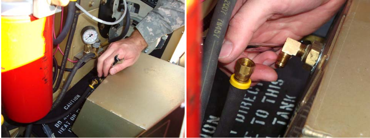
Figure 6. Remove External Fuel Hose from Fitting.
