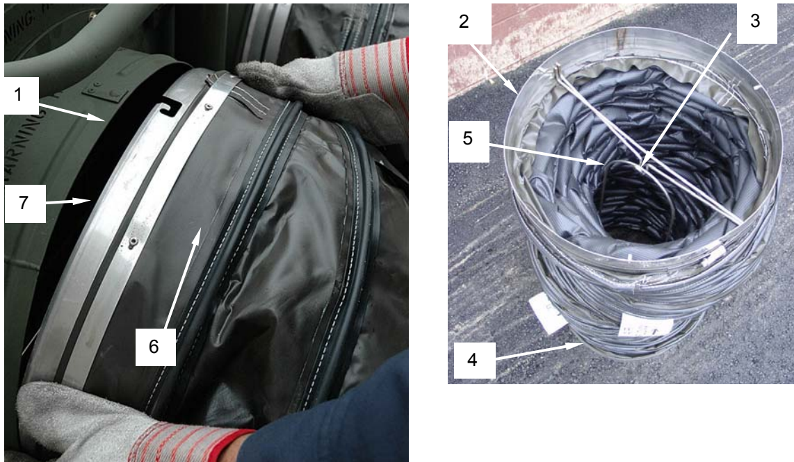
Figure 19. Stowing the Flexible Inlet and Outlet Ducts.
