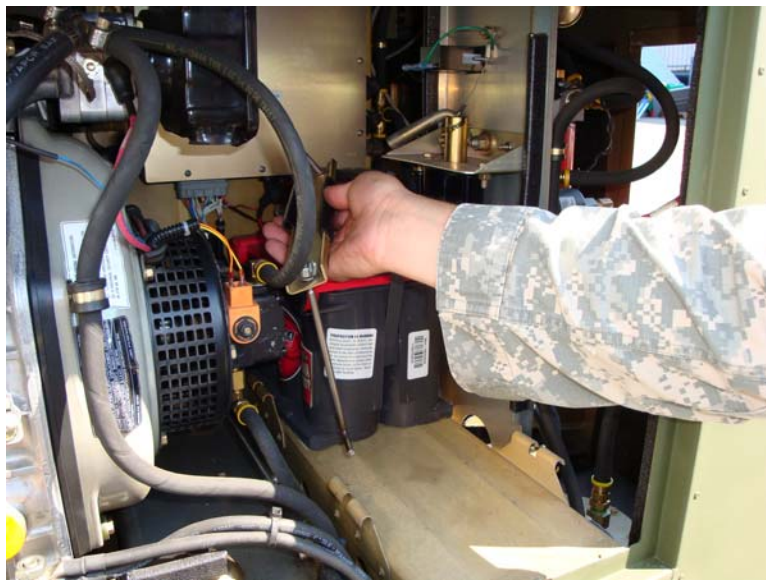
Figure 49. Install Battery Hold-down Bracket on Battery Farthest from Access Door.
