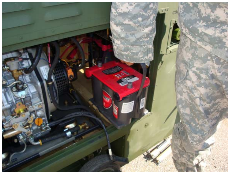
Figure 10. Remove Battery Farthest from Access Door.
