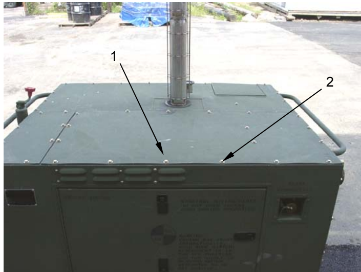
Figure 1. Remove the Top Engine Compartment Cover.
