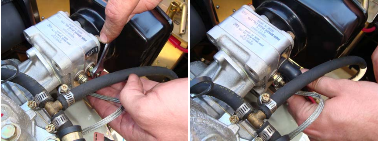
Figure 38. Install Wire to Threaded Stud Labeled GP1.
