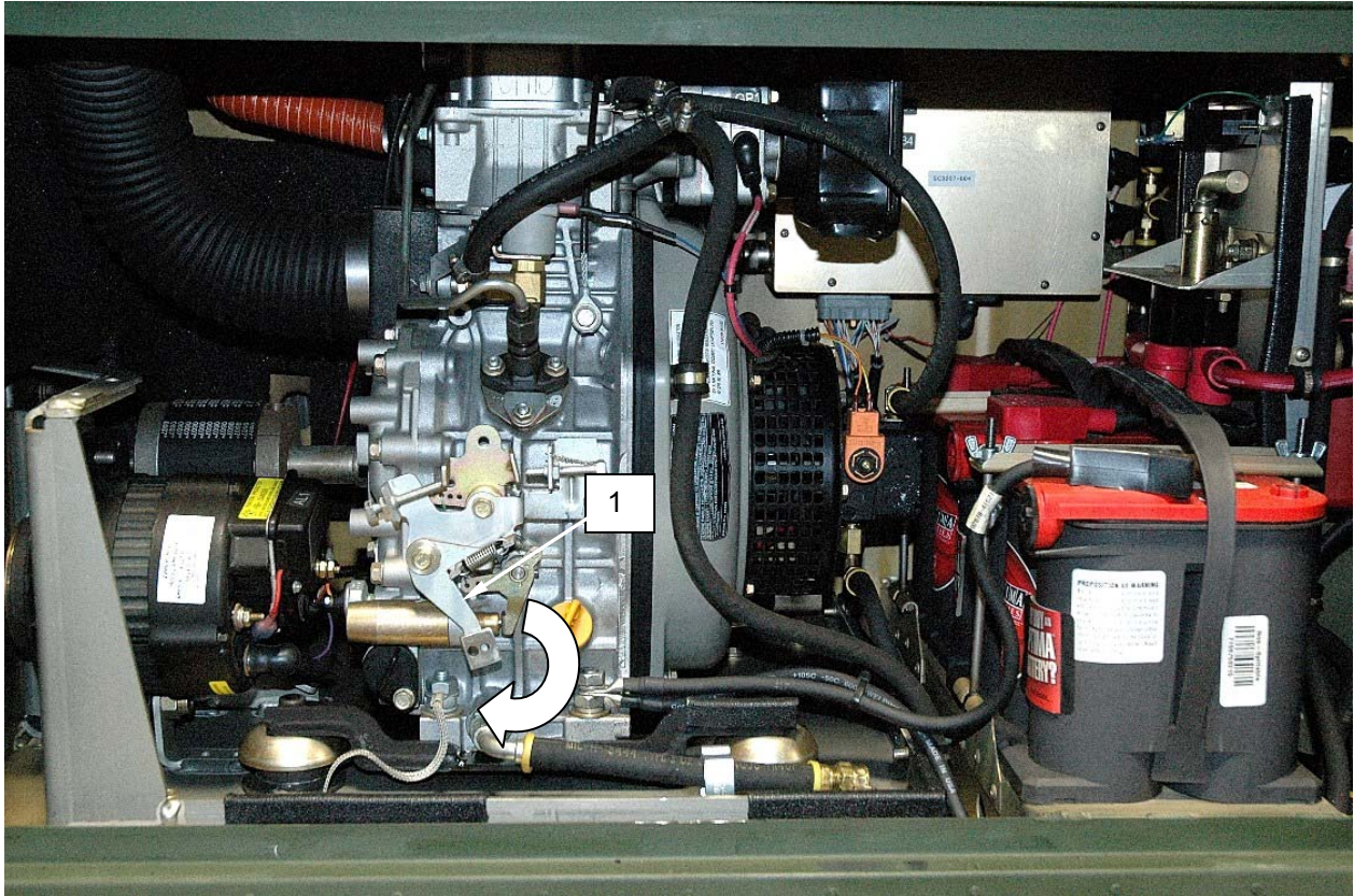
Figure 2. Pull and Hold Engine Stop Lever Until Engine Stops.
