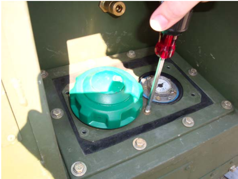
Figure 13. Install Hardware to Secure Retaining Plate.
