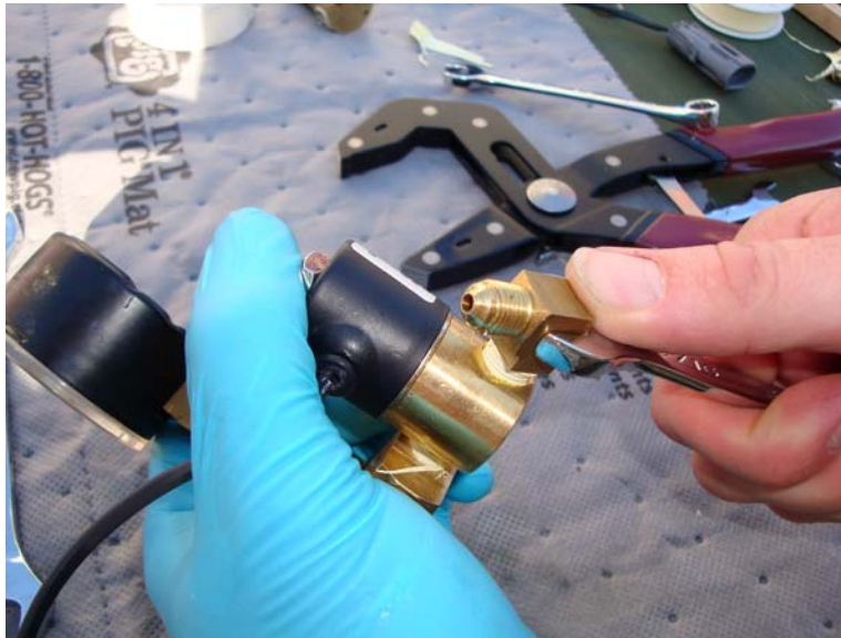
Figure 16. Apply Thread Sealant and Install Elbow Fitting on Solenoid Valve.
