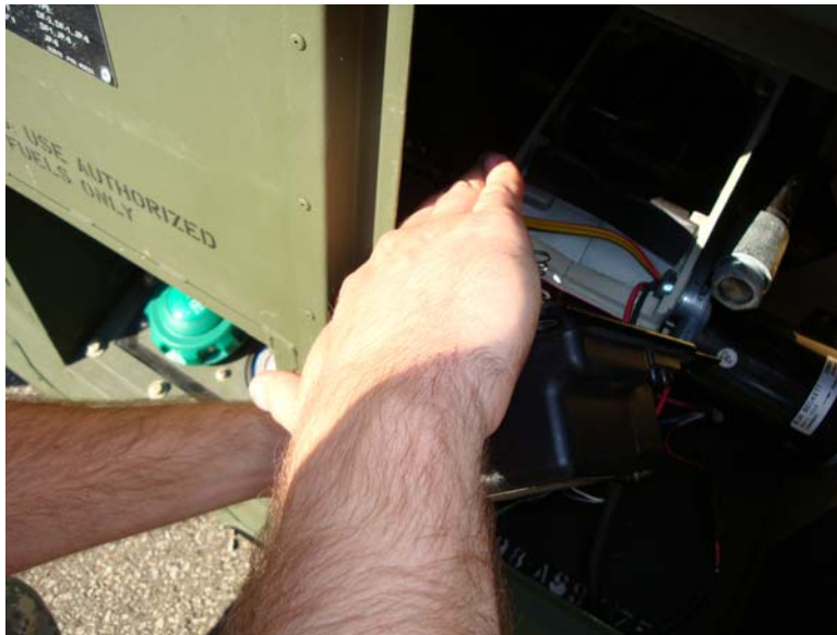
Figure 10. Block Light from Flame Sensor.
