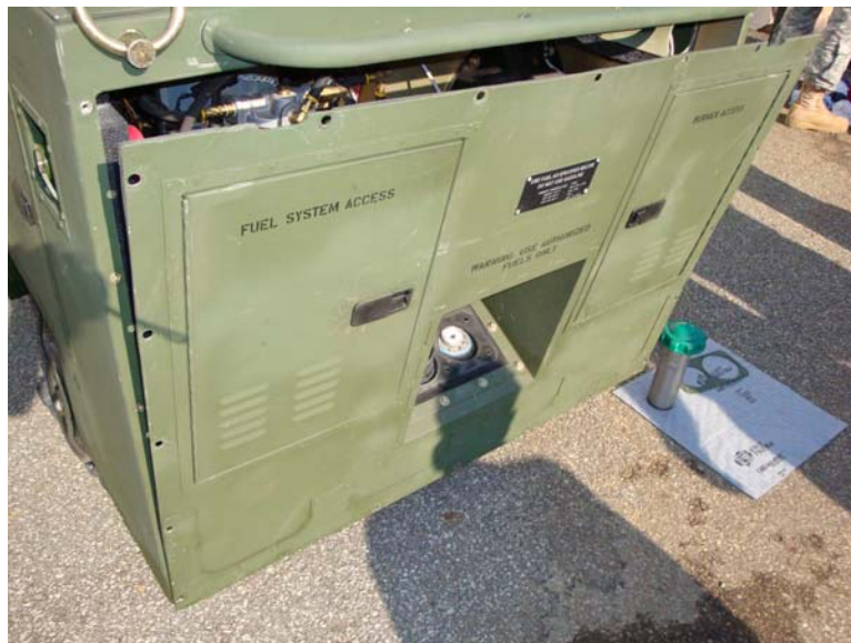
Figure 5. Move End Panel from Heater to Gain Access to Fuel Hose.
