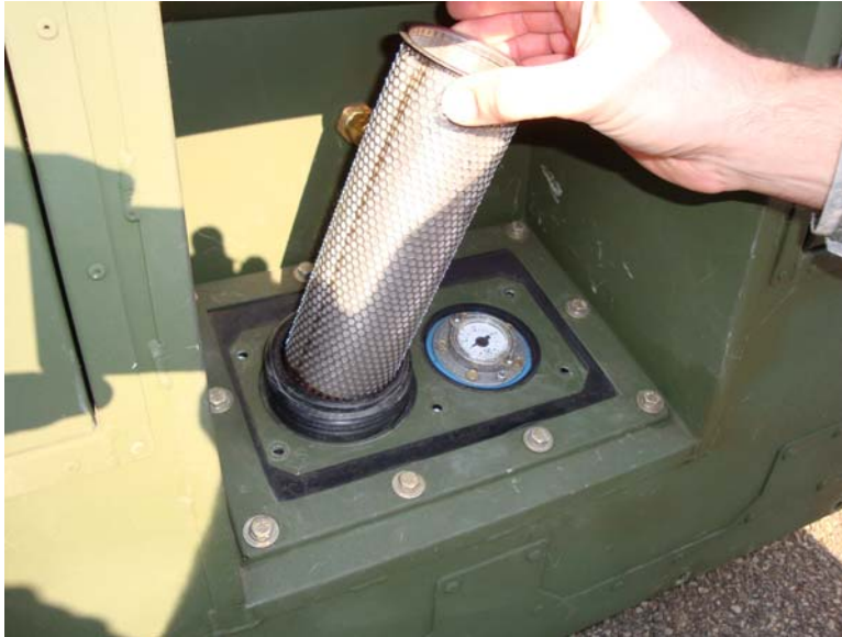
Figure 2. Remove Fuel Filler Cap and Strainer.
