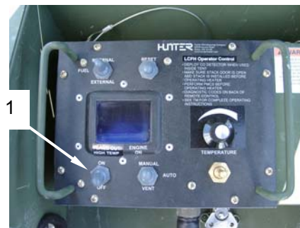
Figure 16. Shutting Down the LCFH Type II.
