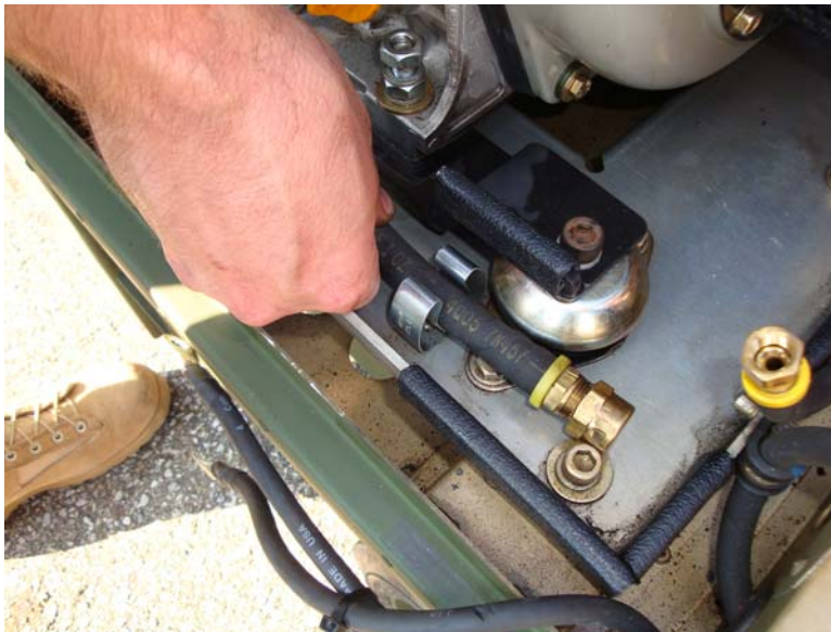
Figure 35. Install Engine Oil Hose in Spring Clamp.
