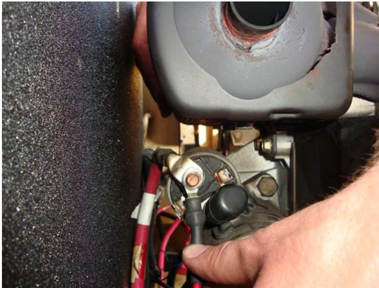
Figure 63. Connect Wires to Starter Solenoid.
