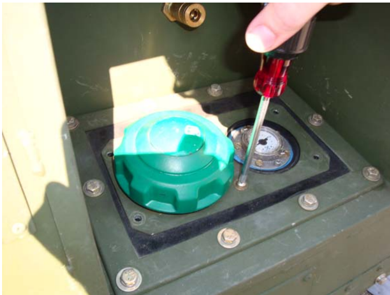
Figure 13. Install Hardware to Secure Retaining Plate.
