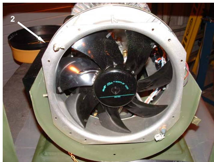
Figure 2. Replace the Electronic Box Assembly, Complete with Wire Harness – Remove the Heated Air Blower.
