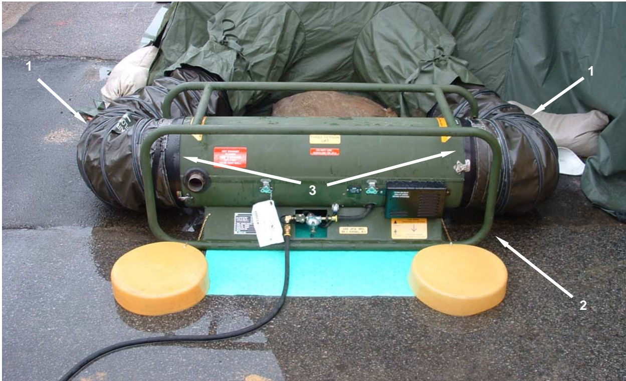
Figure 12. Prepare for Movement – Release Ducts.
