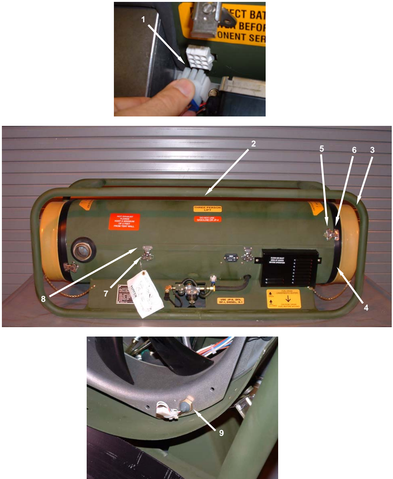
Figure 1. Replacing Flame Sensor.
