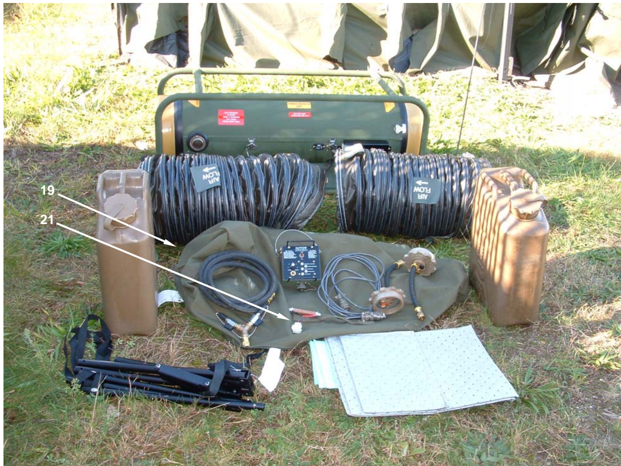
Figure 3. Space Heater Convective (SHC) 60K BTU External Components – Accessory Bag and Components
