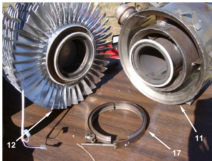
Figure 2. Remove Thermoelectric Generator (TEG) – Continued.
