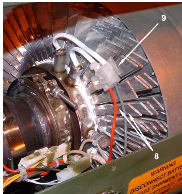
Figure 5. Replace Fin Temperature Sensor – Disassembly.
