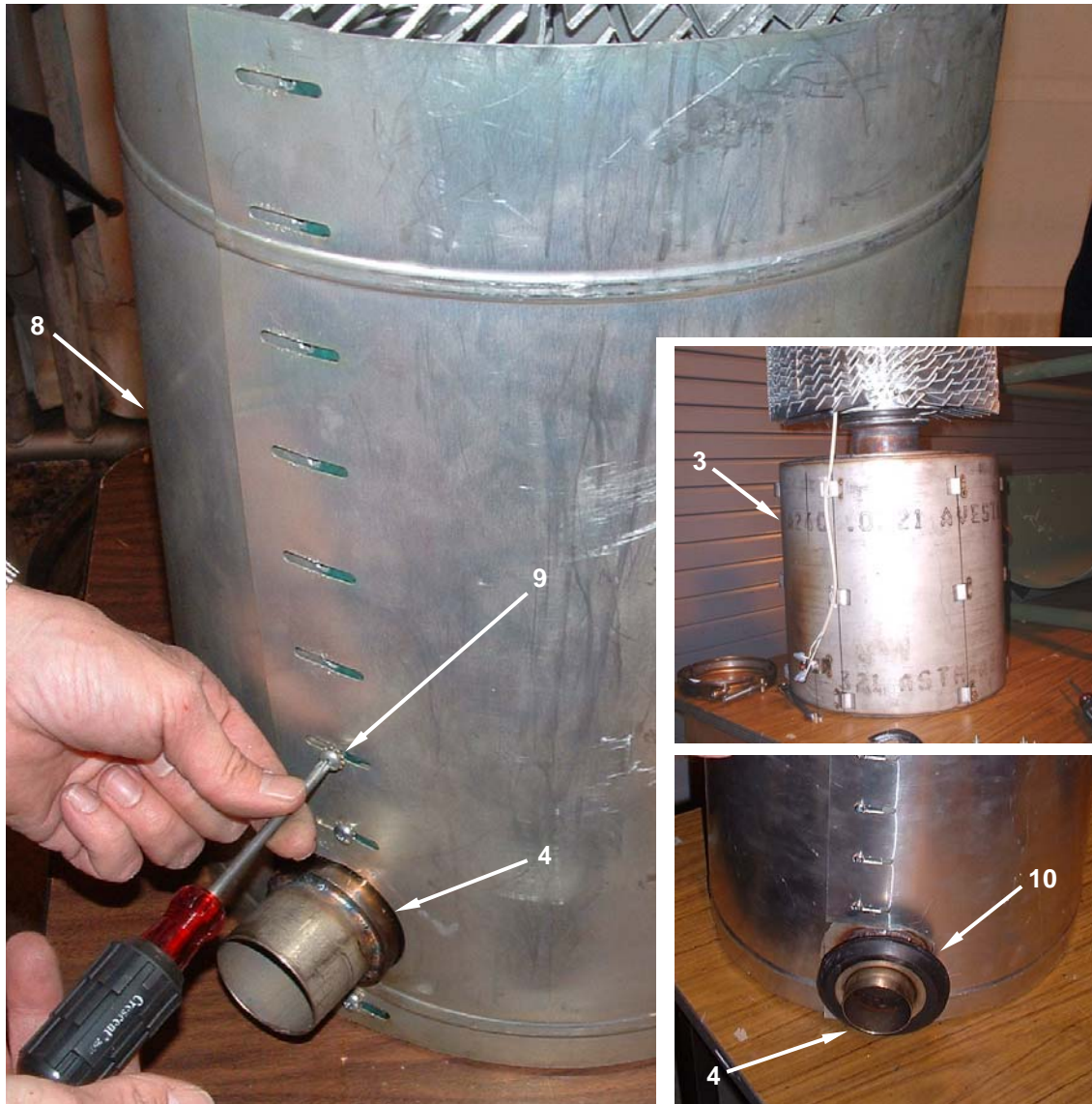
Figure 14. Install the Thermoelectric Generator – Install Wrap Cover.
