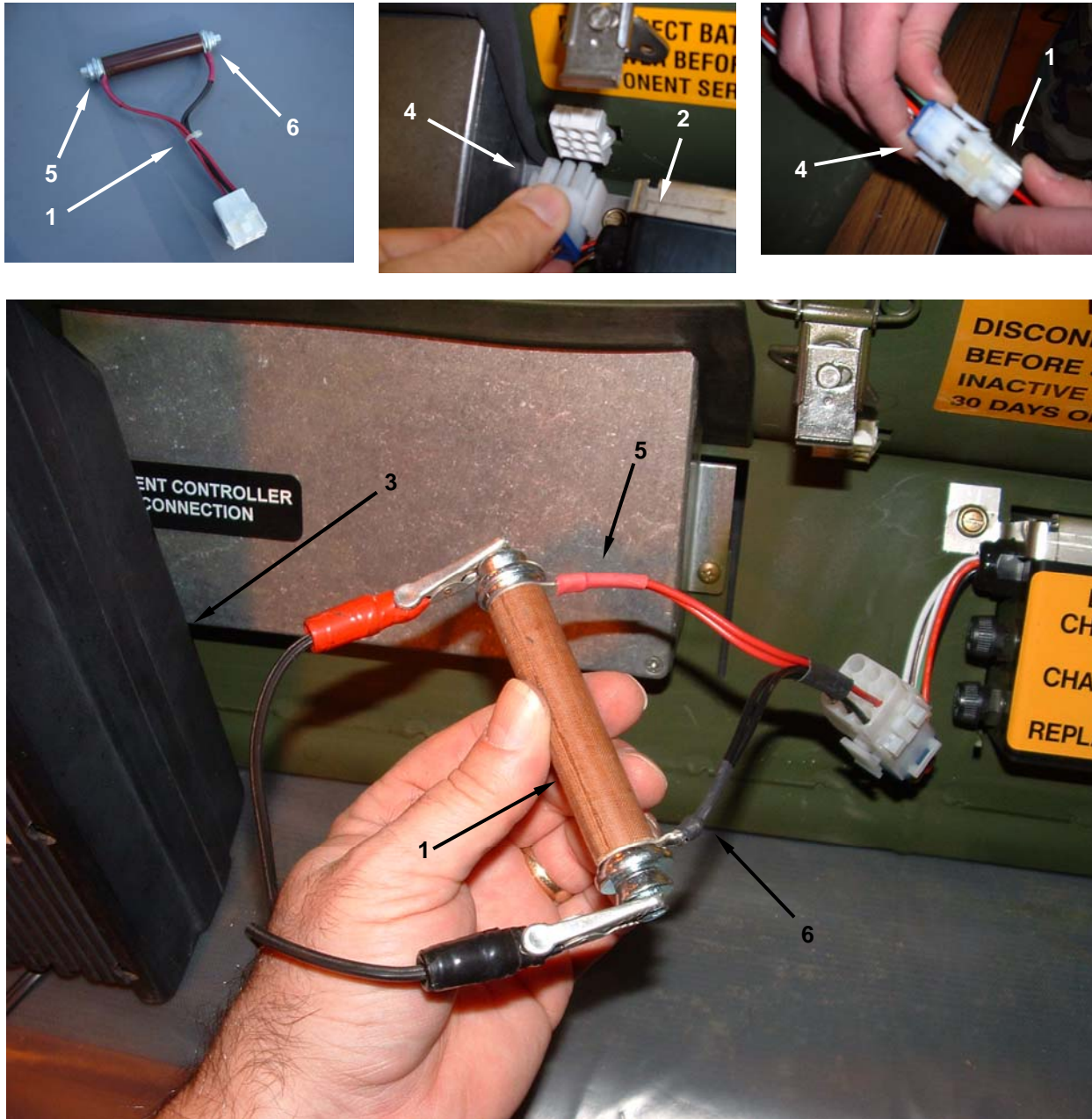
Figure 5. Charging the Battery with an External Charger - Continued.
