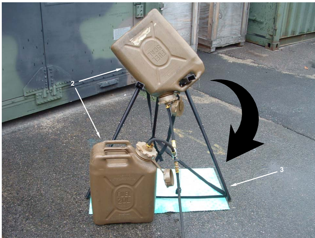
Figure 14. Prepare for Movement – Remove Fuel Cans.
