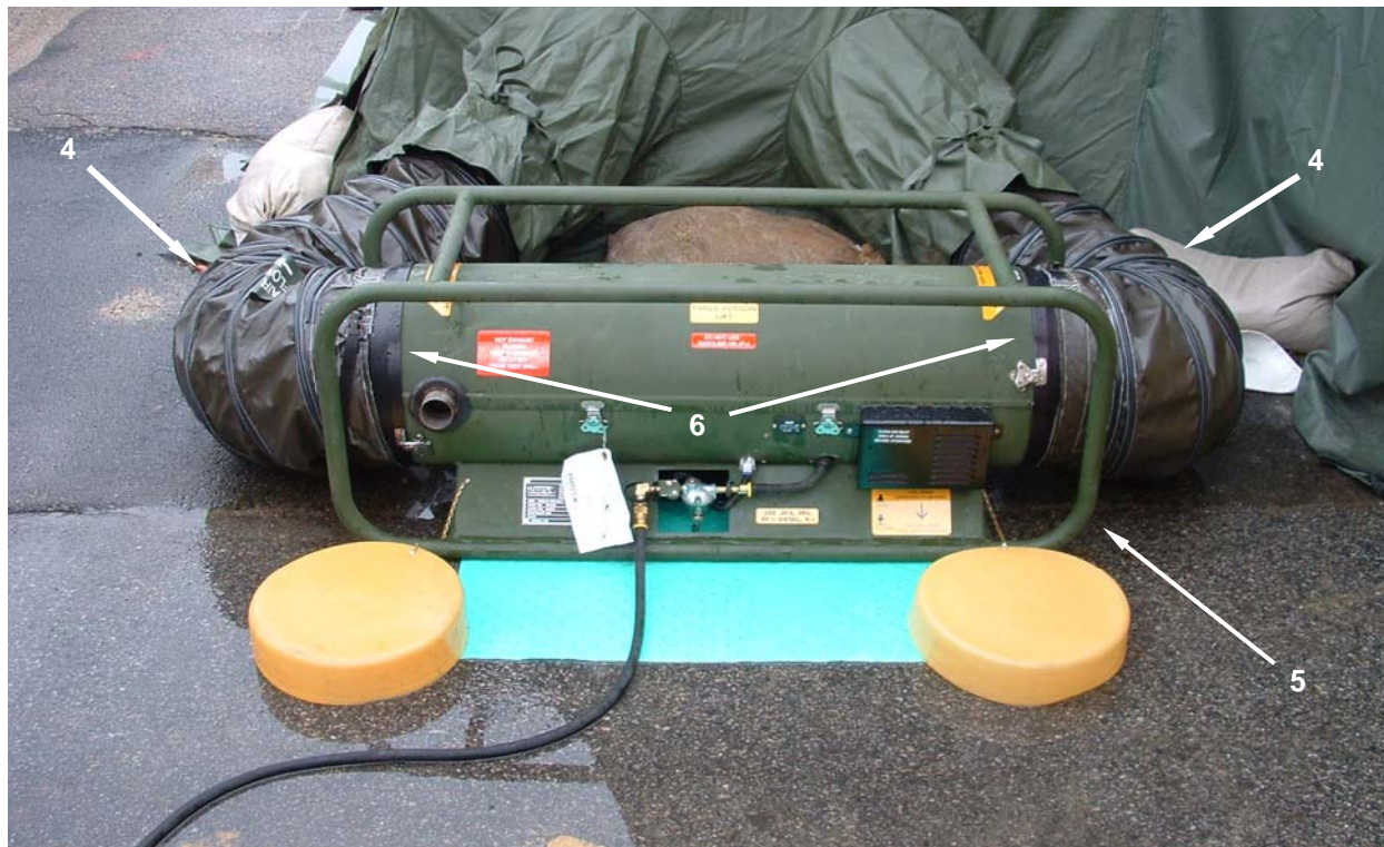
Figure 15. Prepare for Movement – Release Ducts.
