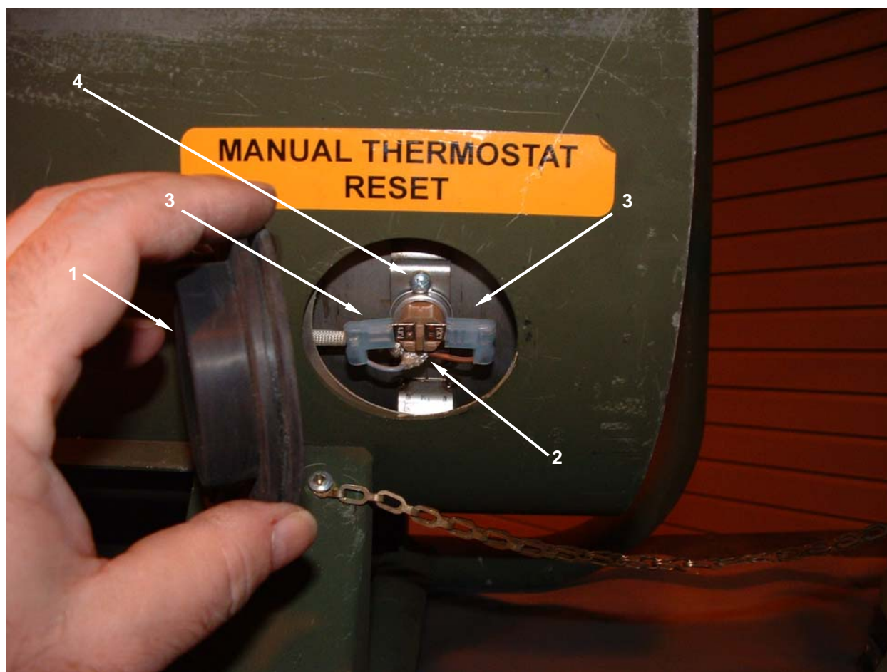
Figure 2. Replace the Manual Thermostat Reset Switch.
