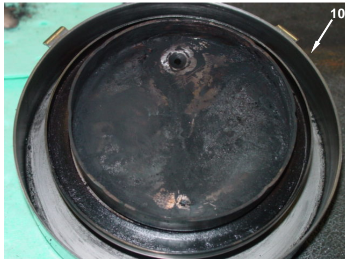
Figure 9. Replace the Burner Assembly Wick - Continued.
