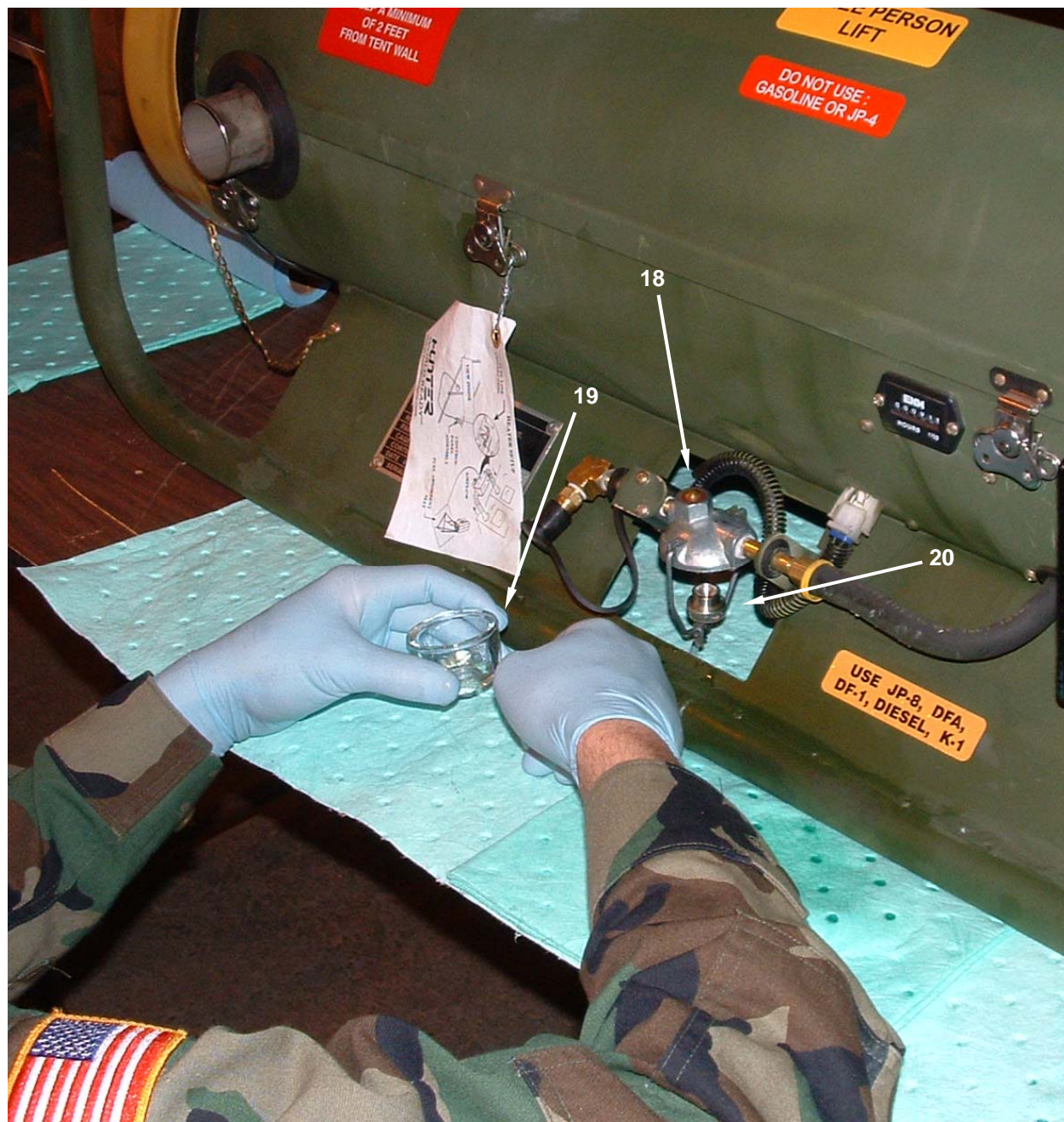
Figure 22. Prepare for Movement – Drain Sediment Bowl (Continued).
