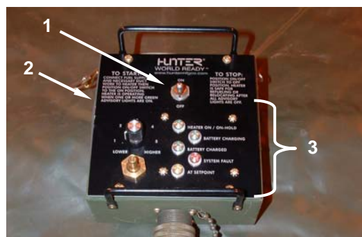
Figure 4. Stopping Heater with In-Tent Controller For Refueling.
