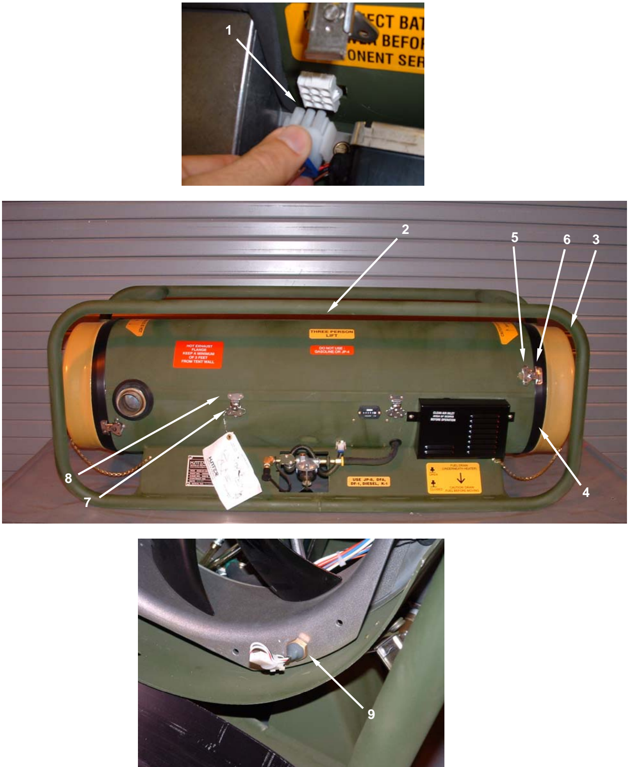
Figure 1. Replacing Flame Sensor.
