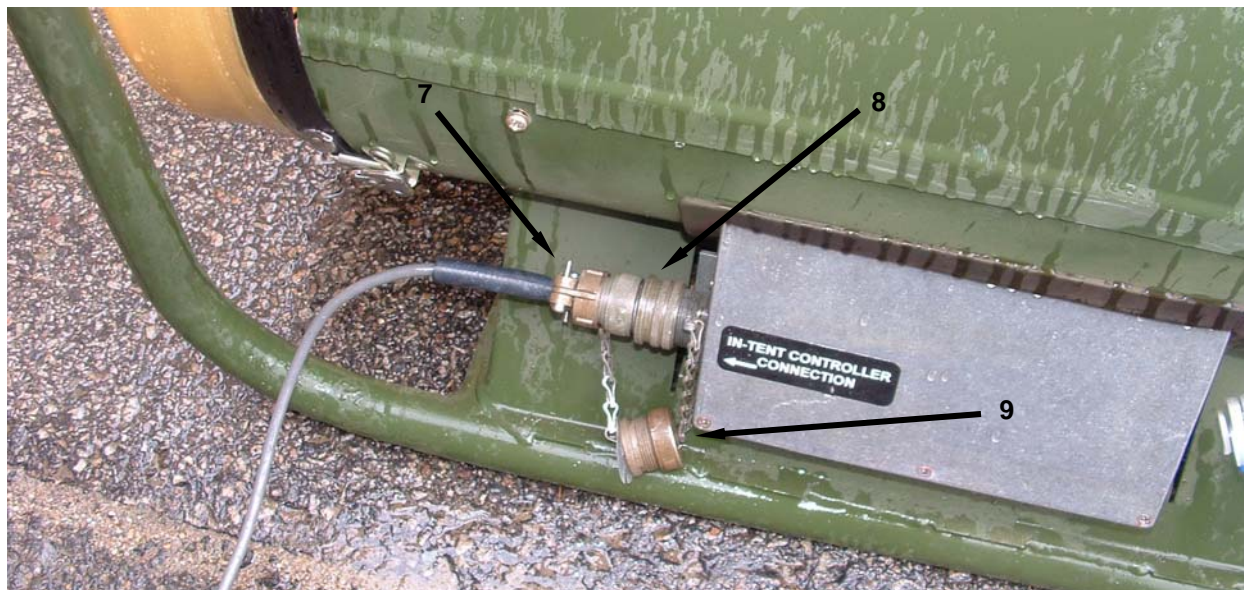
Figure 16. Prepare for Movement – Disconnect the In-tent Controller Cable.
