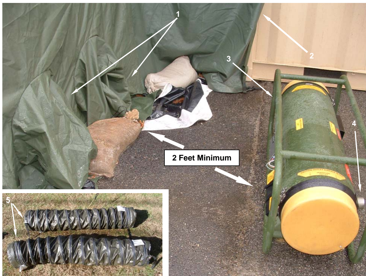
Figure 8. Positioning Heater Outside of Tent.
