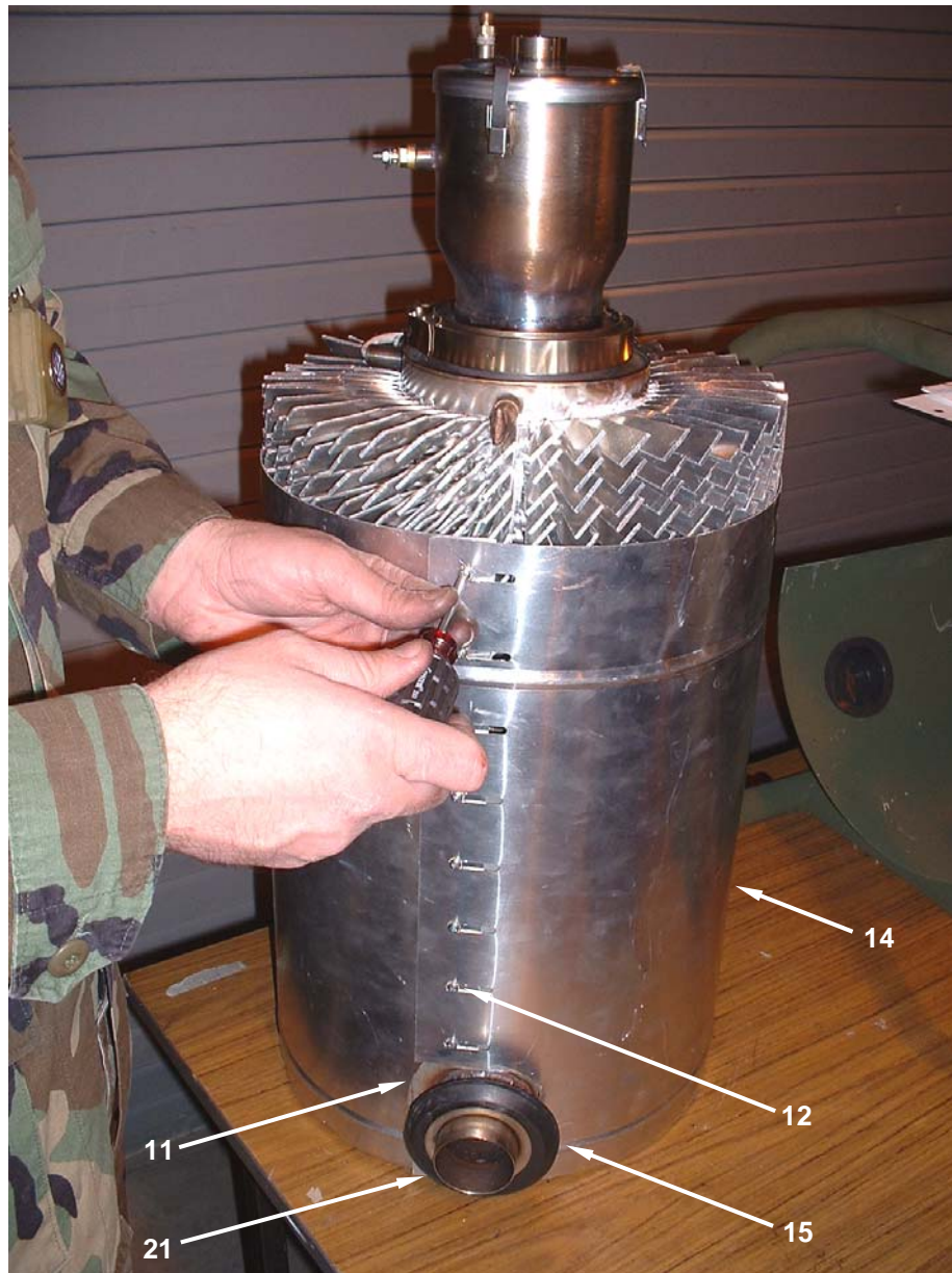
Figure 8. Replace Fin Temperature Sensor – Install Wrap Cover.
