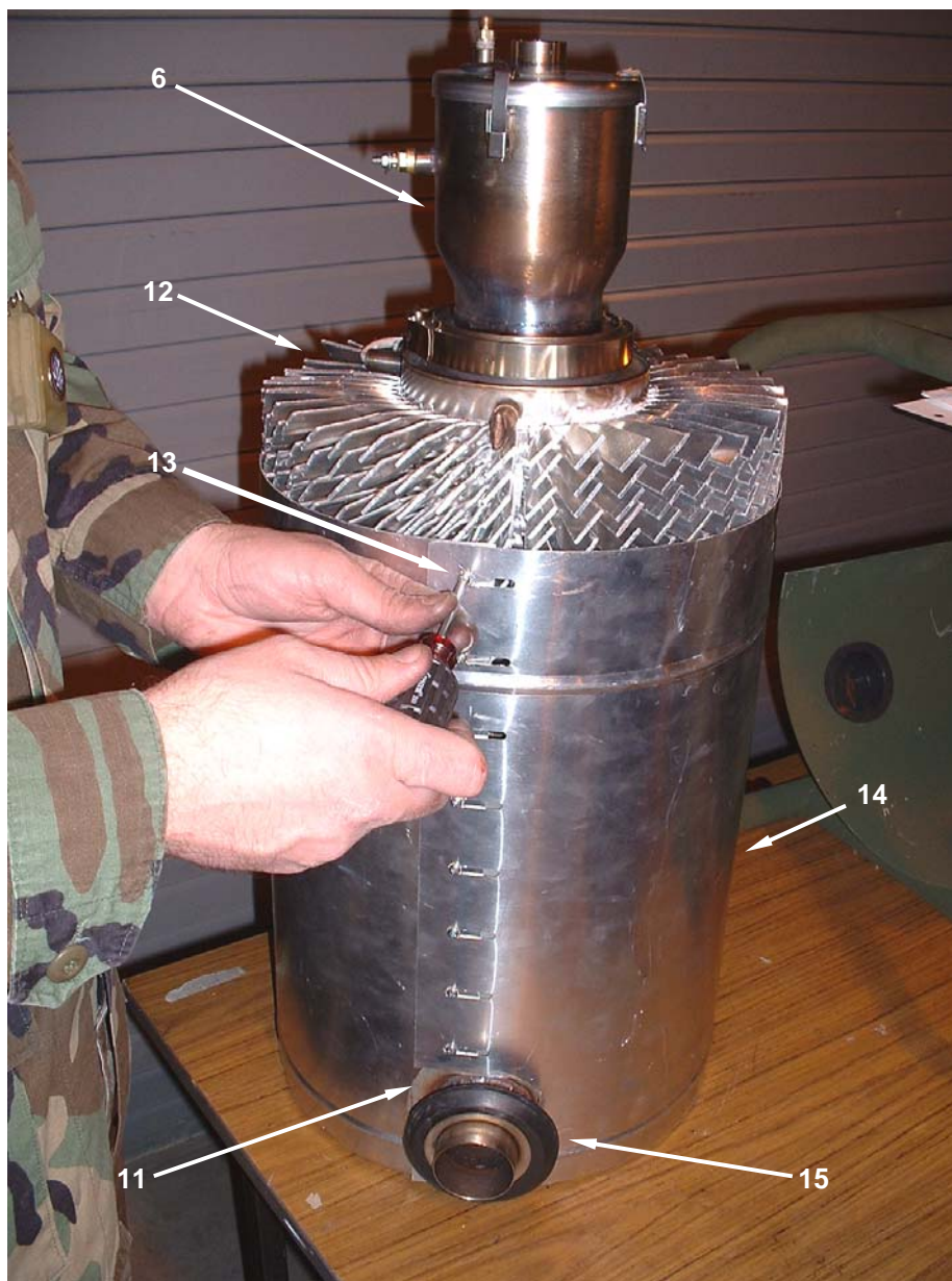
Figure 6. Replace Fin Temperature Sensor – Remove Wrap Cover.
