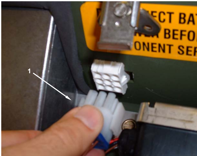
Figure 13. Prepare for Movement – Disconnect Battery.
