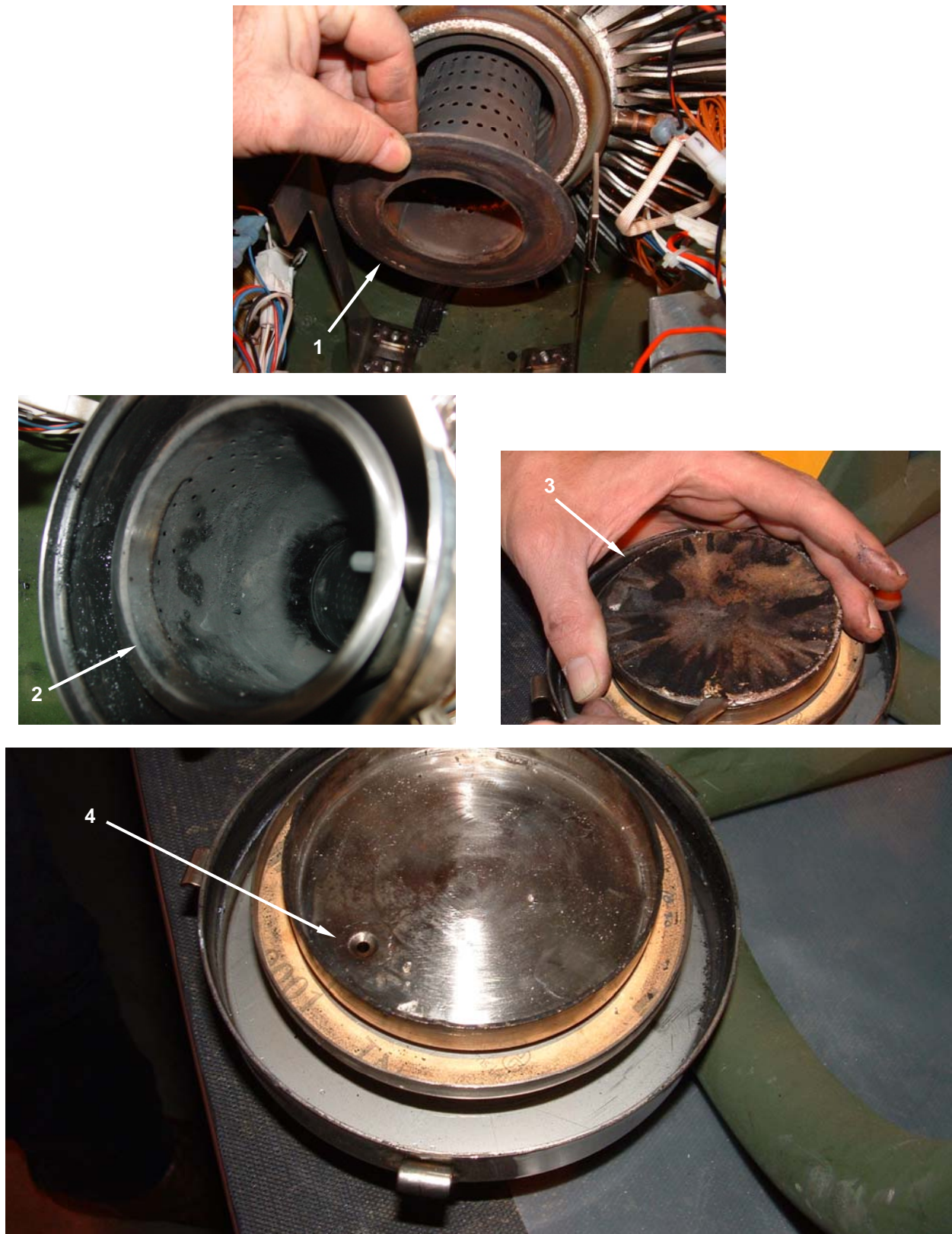
Figure 3. Inspect Burner Assembly.
