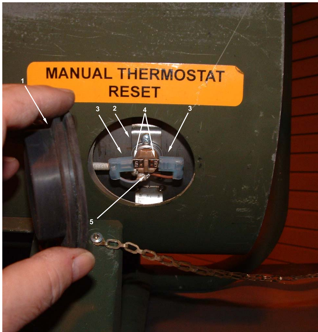
Figure 1. Test the Manual Thermostat Reset Switch.
