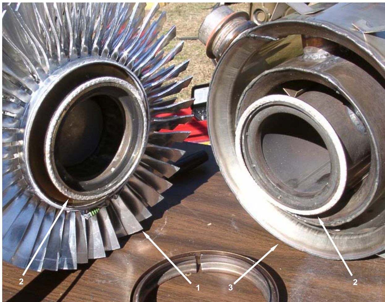
Figure 11. Install the Thermoelectric Generator – Install Fiberglass Rope.
