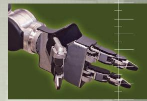
Because it was designed as a "hand" rather than a claw, the MK-1 can use many hand tools made for a human hand, including shovels, drills, hammers and more. In addition, its "palm" adds strength and stability, also allowing objects to be lifted from below rather than simply grasped from above. And its force-feedback system means that operators can virtually feel what they're grasping, making it possible to lift a fragile egg safely, or hoist 155 mm projectile with ease.
