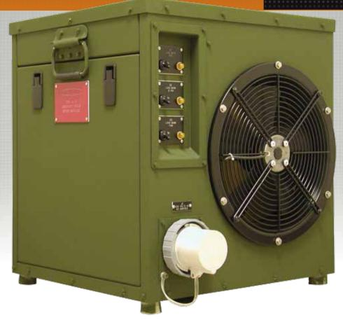
HDT's ruggedized 15 kW and 30 kW portable load banks simulate the electrical loads to power sources such as generator sets that may be encountered in military and heavy industrial applications. The load banks use their energy output to test, support or protect those power sources.
