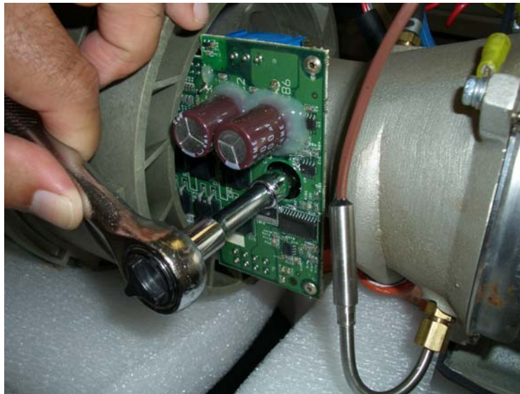
Figure 5.6-7 Bolt Removal Detail, Vent Fan Assembly
